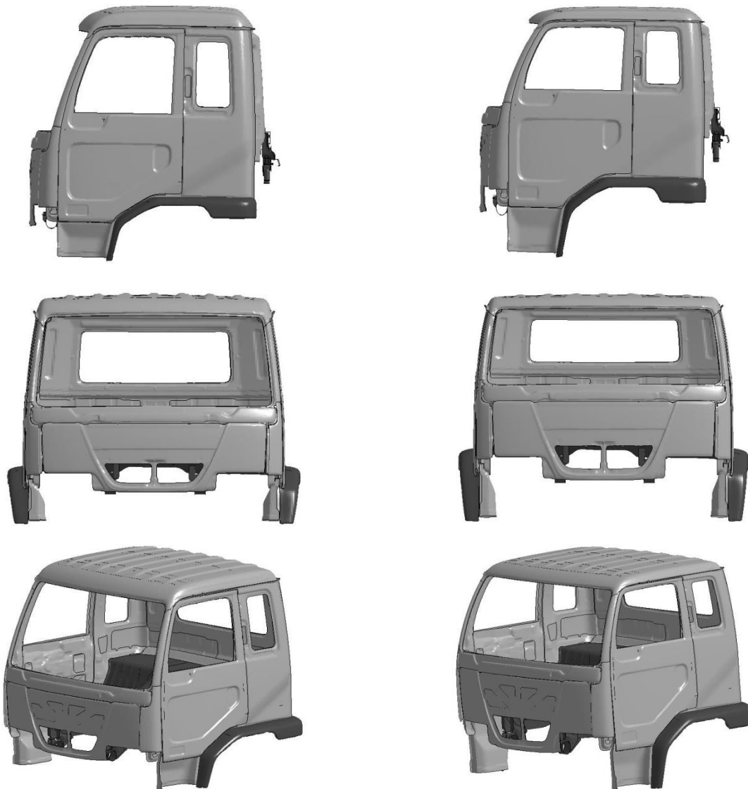
Figure 10-1 Original COE DoS cabin vs. morphed conventional cabin models.
