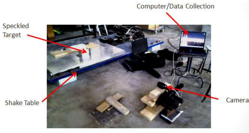
Figure F-1: Lab testing setup using a shake table with a known displacement.
