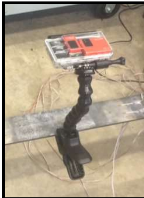
Figure 71: Assembled GoPro® DIC sensor for 3D strain collection
