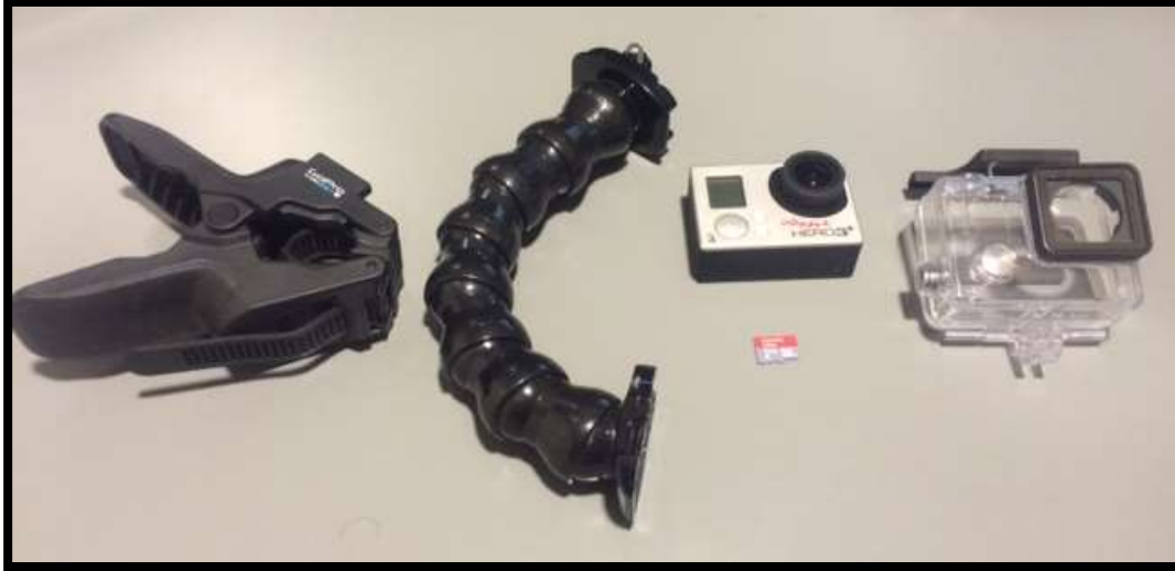
Figure 68: The collection of parts necessary for assembling the 2D GoPro® DIC sensor
