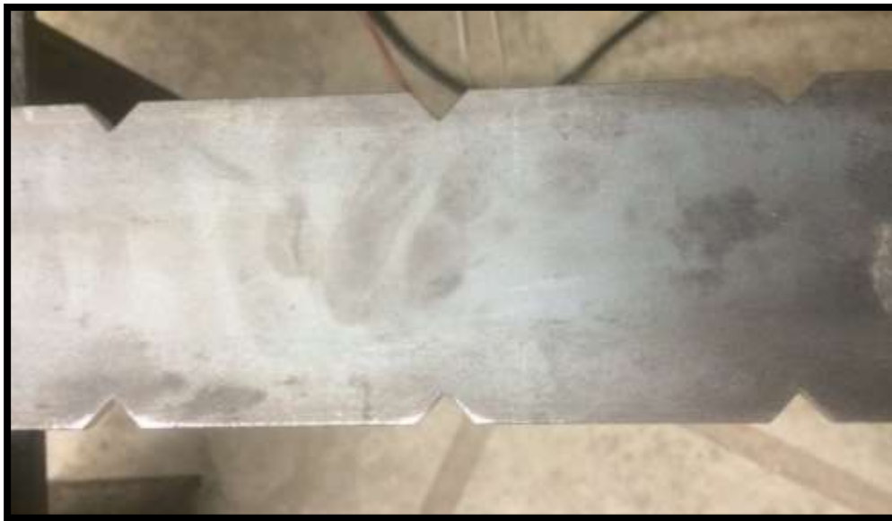
Figure 73: Photo showing the machined notches on one side of the test beam
