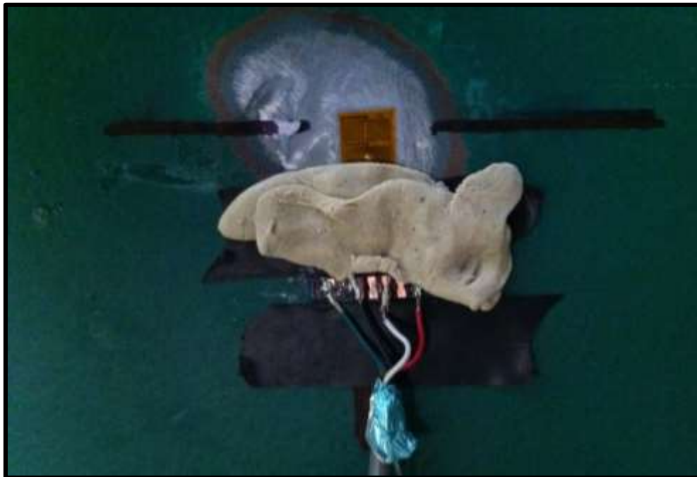
Figure G-1: Photograph of Full Bridge Strain Gauge Installed on the Bottom Flange of Beam D, South Face
