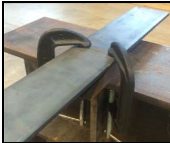
Figure 76: Picture displaying the clamps used to create fixed conditions for the supports of the test apparatus
