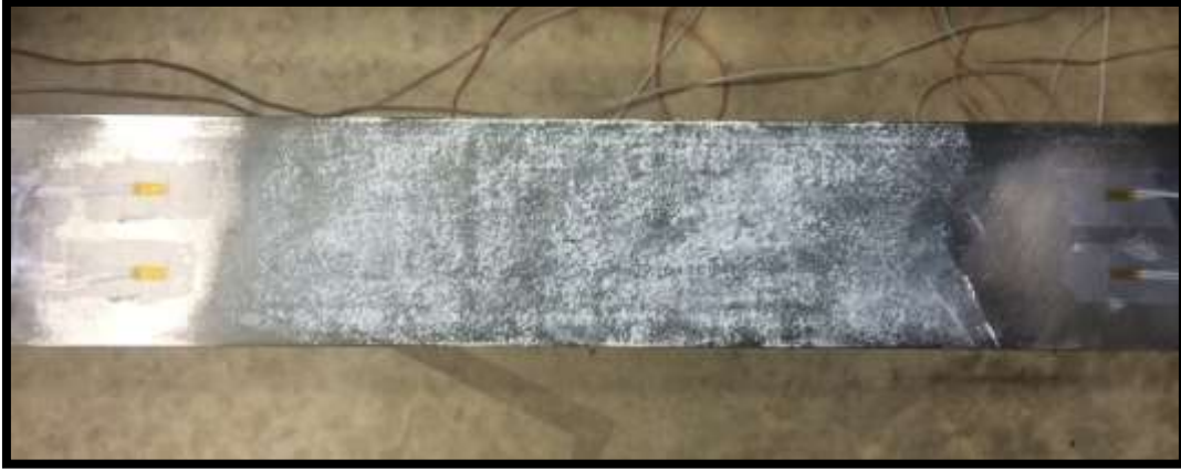
Figure 78: Top-down view of the test apparatus showing the placement of the foil gauges on either side of the speckle pattern on the center span
