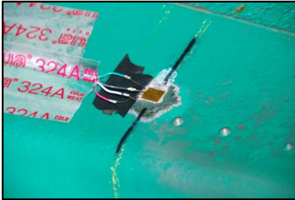
Figure G-9: Photograph of Full Bridge Strain Gauge on the Top Flange of Beam E, North Face
