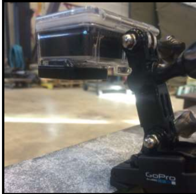
Figure K-9: Experimental DIC sensor that tests the short range capabilities of the GoPro® camera
