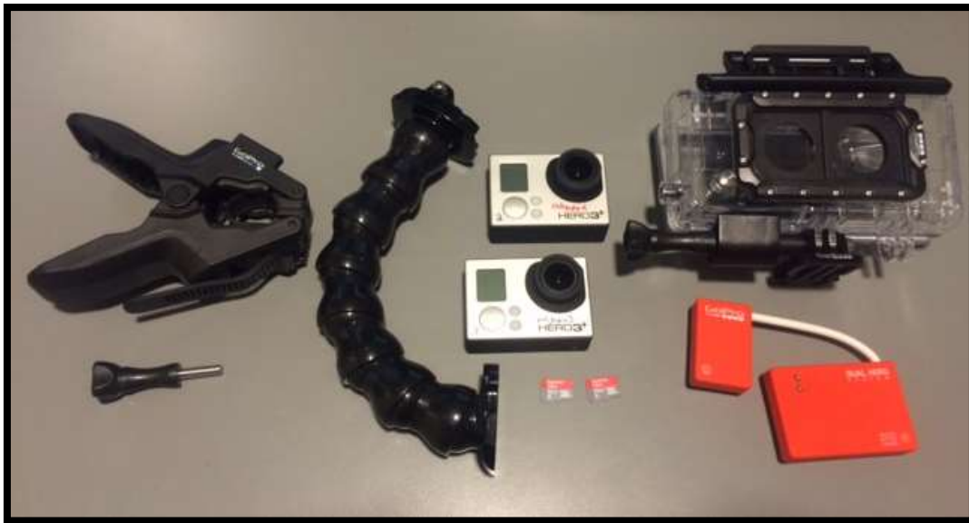
Figure 70: The collection of parts necessary for assembling the 3D GoPro® DIC sensor
