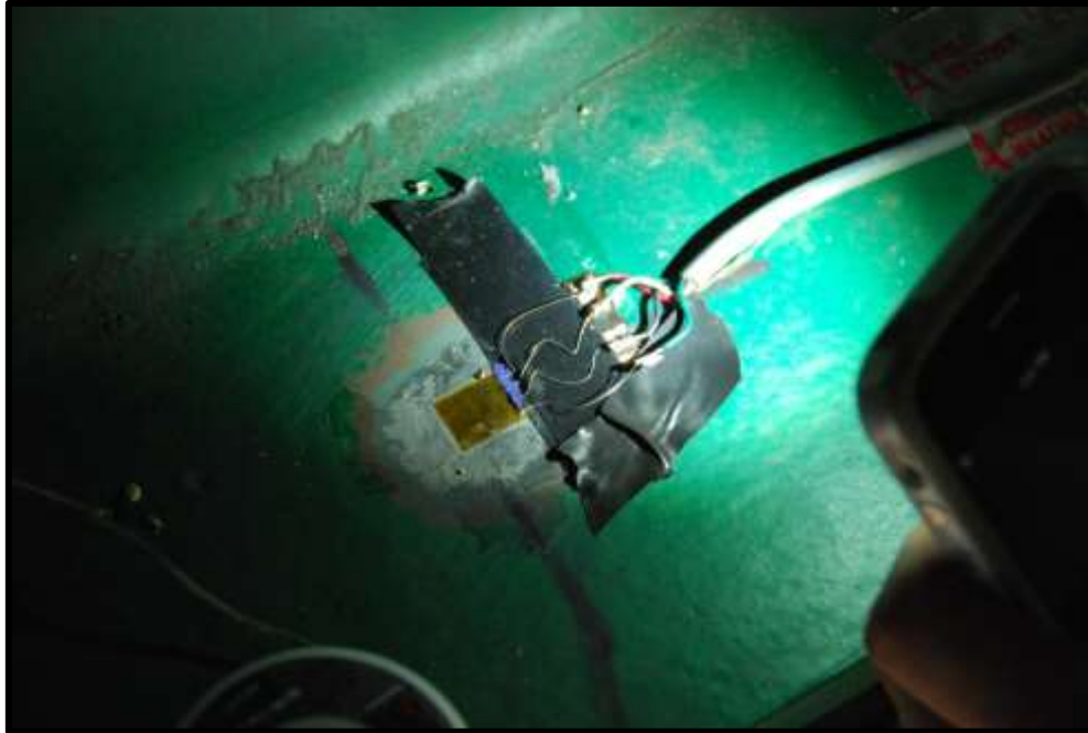
Figure G-1: Photograph of Full Bridge Strain Gauge Installed on the Bottom Flange of Beam D, South Face
