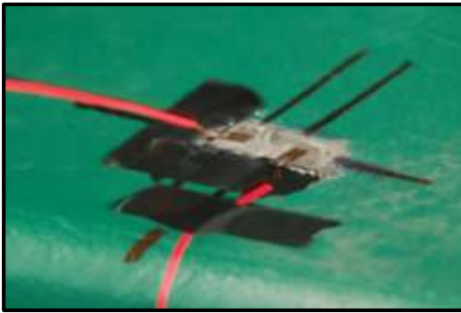
Figure C-20: Photo of Gauge Installation – Quarter Bridge Gauges
