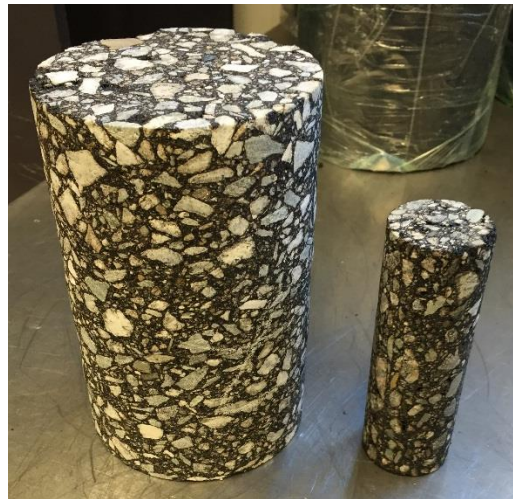
Figure 2.5 Comparison of standard size (left) vs. small geometry specimens (right)
