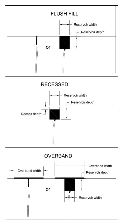
Figure 12. Crack sealing and filling configurations.
