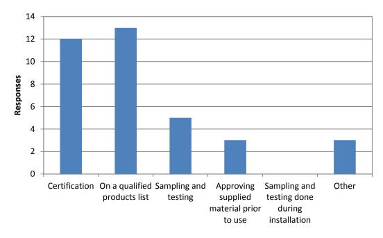
Figure 10. Survey responses of methods of evaluating material in the field to verify that the proper sealant was used.
