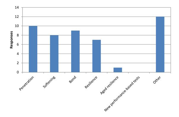
Figure 9. Material acceptance tests from survey responses.
