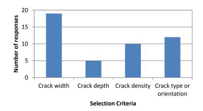
Figure 1. Selection criteria for crack sealing from survey responses.
