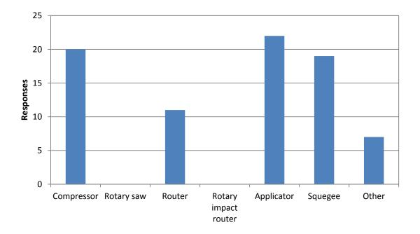
Figure 13. Typical equipment used in the crack sealing process from survey responses.
