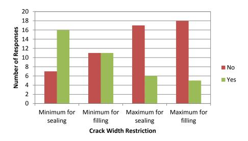
Figure 2. Policy restrictions on crack width for filling and sealing from survey responses.
