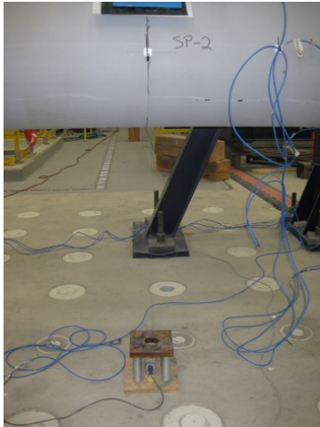
Figure 7: Vertical Deflection Measurement
