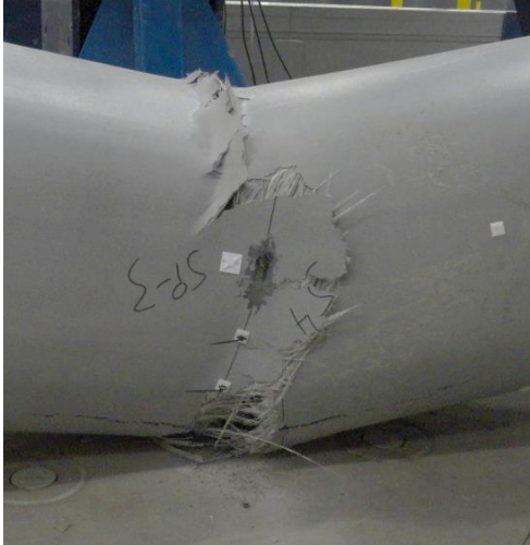
Figure 31: Tension Failure of Pile E-4FB
