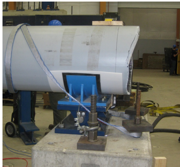
Figure 2: Saddle and Support Configuration
