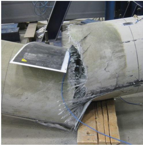
Figure 25: Tension Failure of Pile A-4FB
