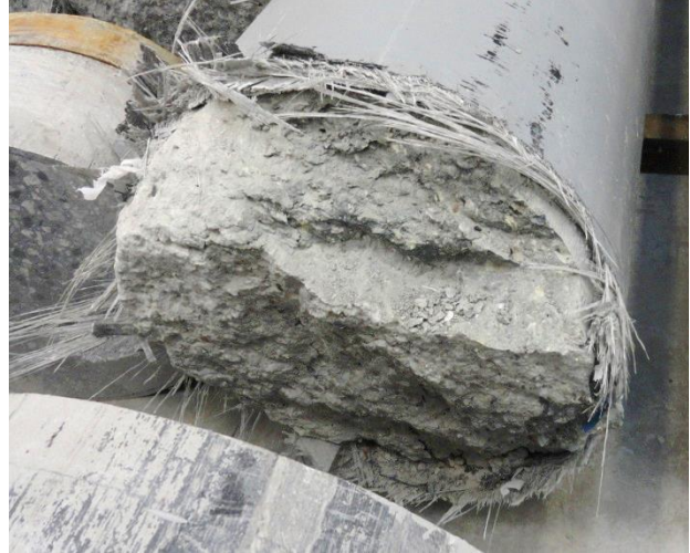
Figure 32: Cut at Failure of Pile E-4FB
