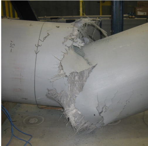
Figure 21: Tension Failure of Pile G-4FB
