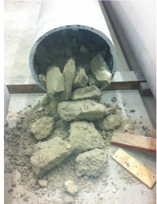
Figure 20: Concrete Plug from Pile B
