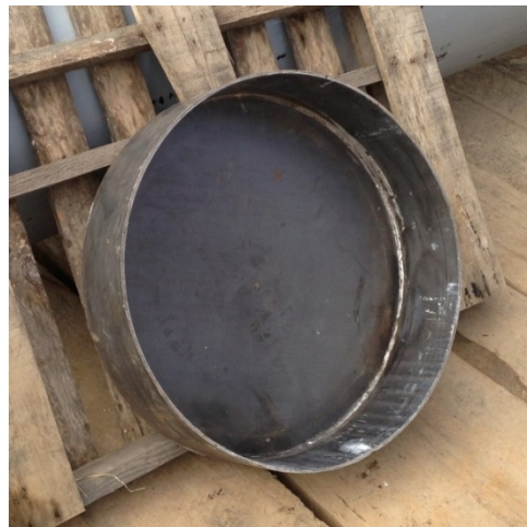
Figure 7: Redesigned Driving Cap for Restrike
