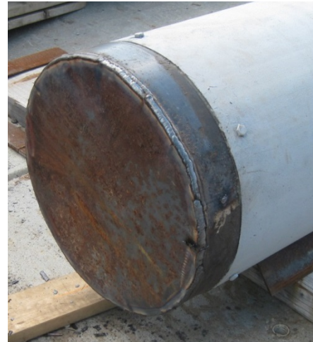
Figure 3: Driving Shoe for Filled Piles
