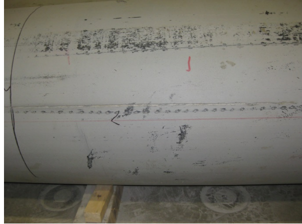
Figure 15: Scratch from 21 to 28 Feet
