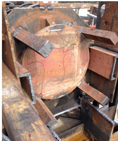
Figure 4: Steel Driving Cap
