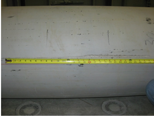
Figure 14: Scratch from 7 to 10 feet
