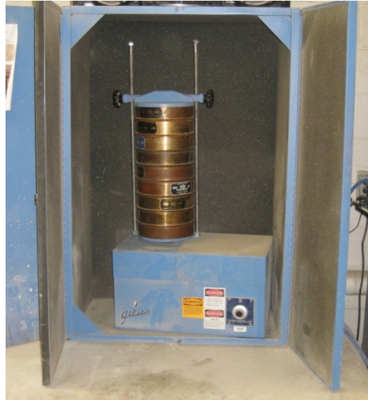
Figure 15: Sieve Shaker for Grain Size Analysis
