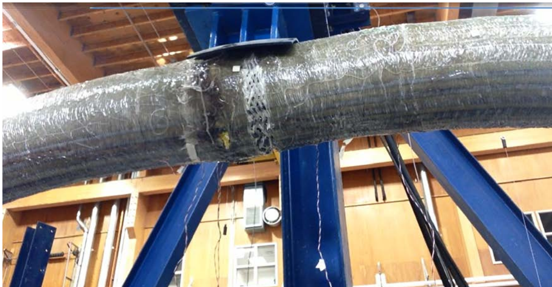
Figure 18 - Arch tensile failure at midspan of shallow arch
