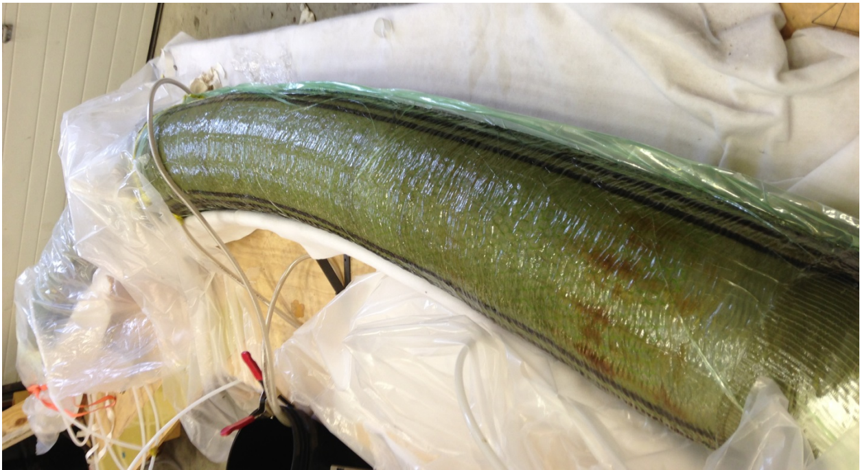
Figure 14- Infused new braid arch
