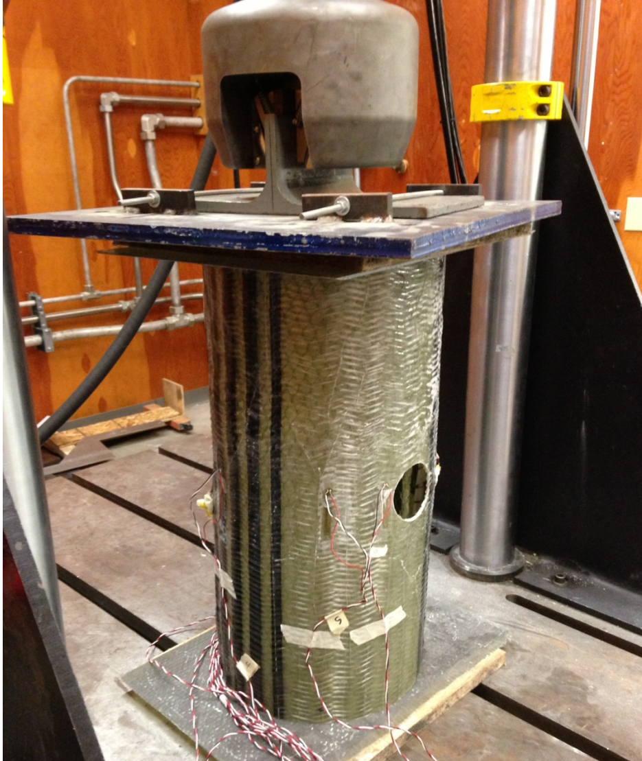
Figure 15 - Specimen during hollow compression testing.
