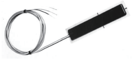
Figure 4.9: Strain gauge (HBP-35-250-06-3VR)
