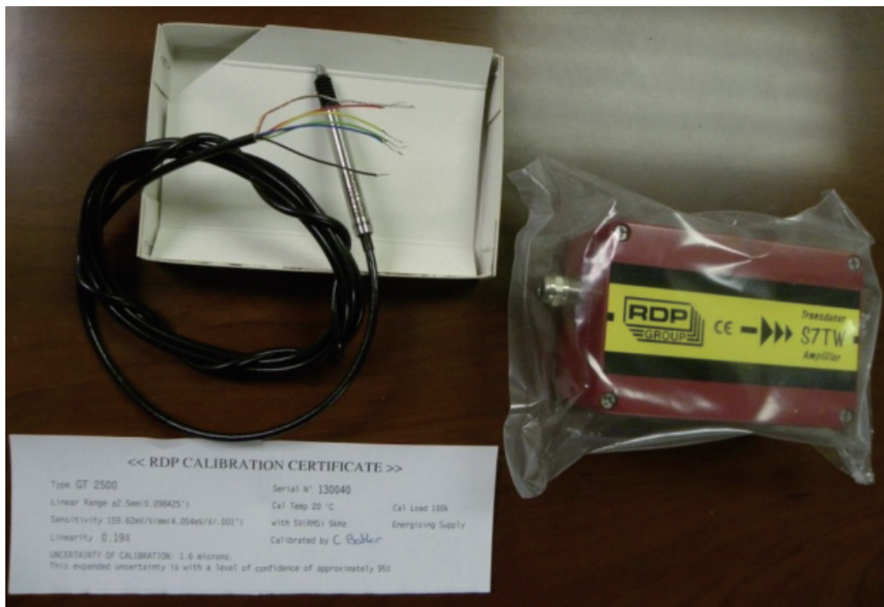
(a) Transducer GT2500 (left) and amplifier S7TW (right)
