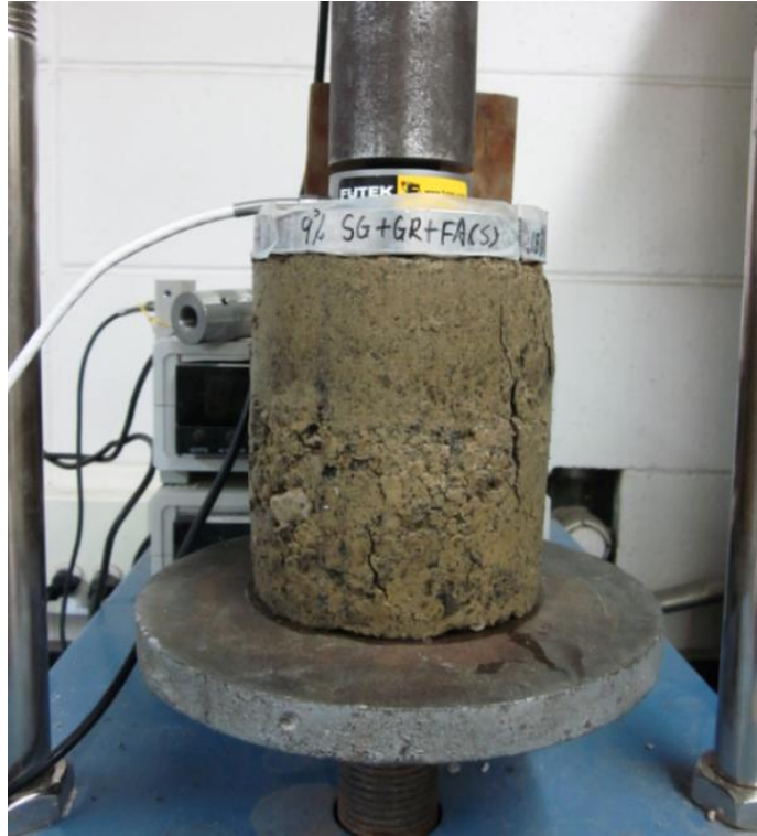
Figure 6. Unconfined compressive strength test on a fly ash-treated soil specimen
