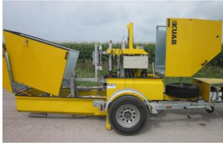
Figure 13. Kuab falling weight deflectometer setup
