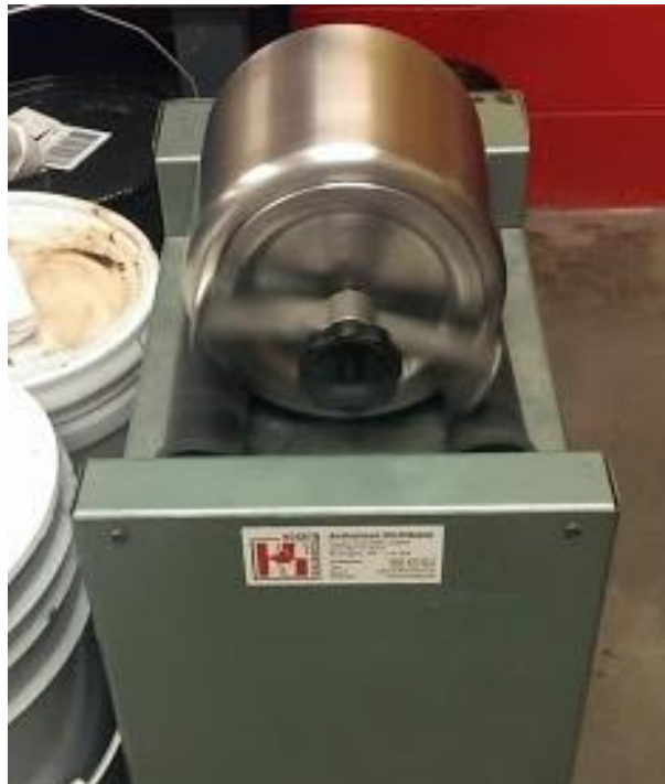
Figure 4. Micro-Deval testing machine used in this study
