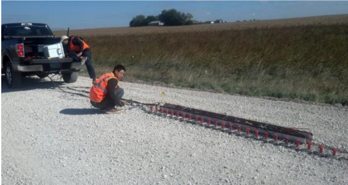
Figure 14. MASW test setup with landstreamer
