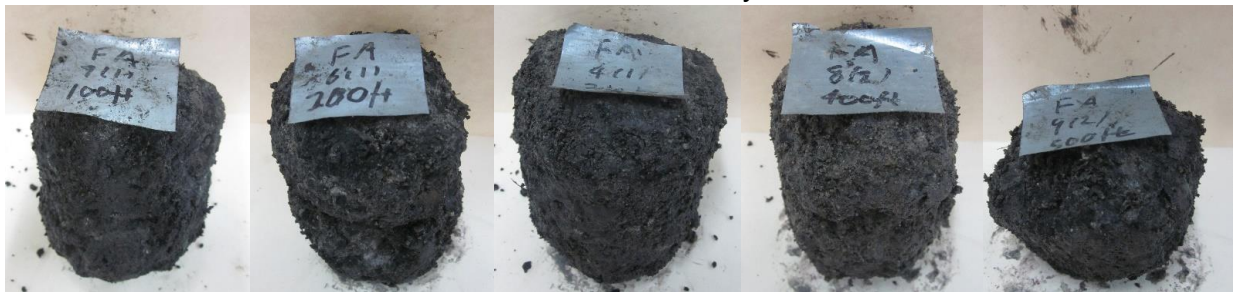
After 3 rd freeze-thaw cycle
