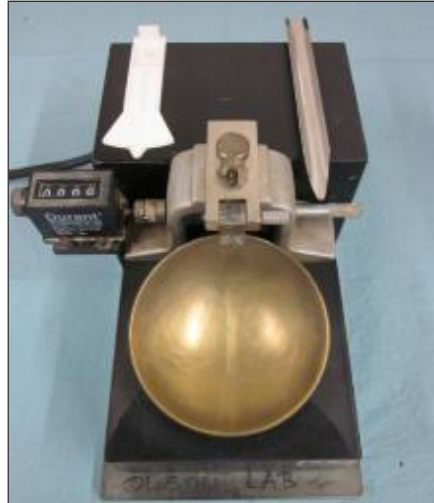
Figure 3. Liquid limit test device used in this study
