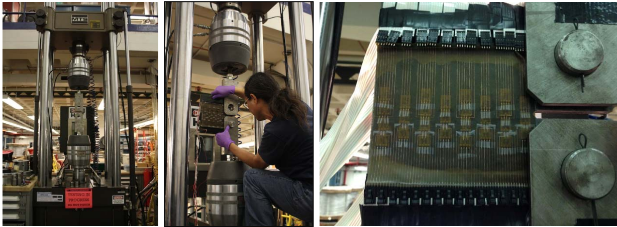
Figure 23. Left: fatigue test setup and test fixture; Middle: installation of specimen; Right: specimen insulated with duct tape, placed into the testing frame, secured with the fixtures, and connected with cables (to the reading unit).
