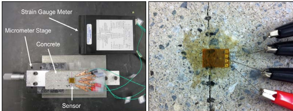
Figure 1. Left: top view of the experiment setup. Right: positioning of the sensor 90^\circ to the crack (source: Tung et al. 2014, see journal papers in Conclusions).
