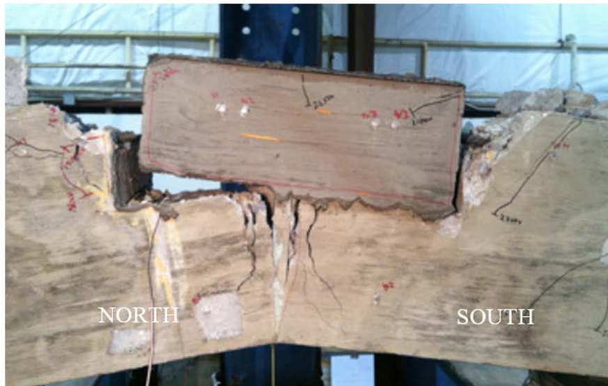
Figure 37. VHPc Pocket in Specimen V-4-5-II Showing Interface Separation and Reinforcing Bars Ruptured
