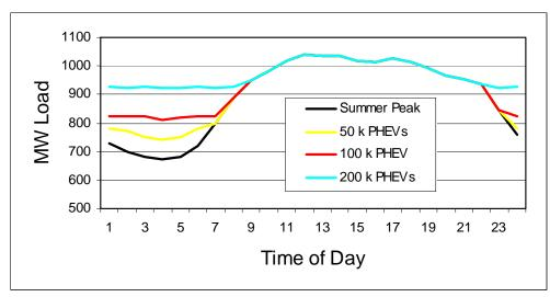
Figure 10: Summer Peak PHEV Load Impacts: Optimal Nighttime Charging
