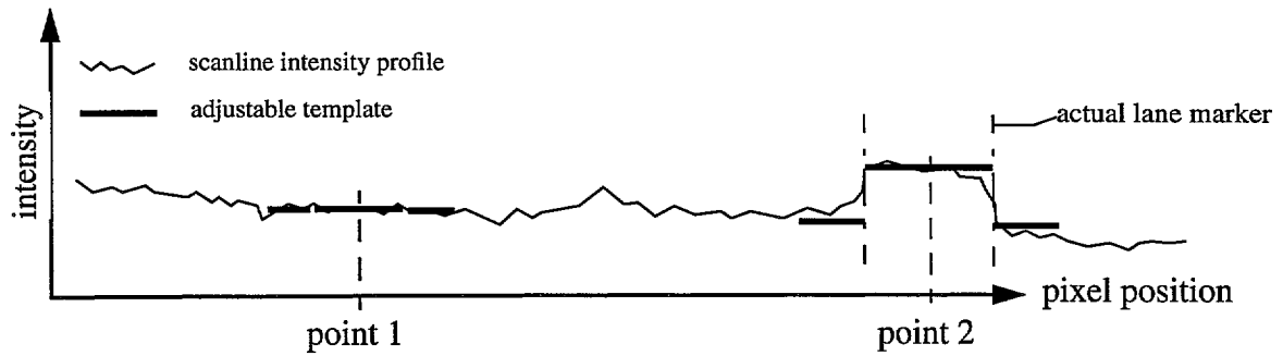
Figure 3-6: Illustration of the adjustable template as a function of pixel position
