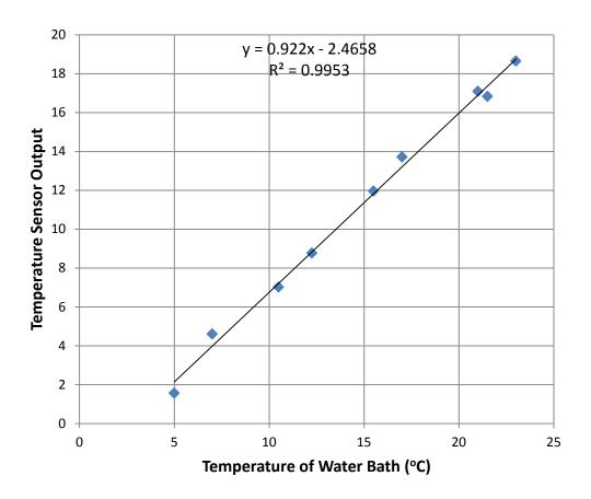
Figure 3.8: Temperature sensor output vs. the temperature
