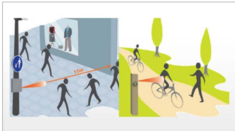
Figure 11 Pyroelectric Sensor Functional Diagrams
