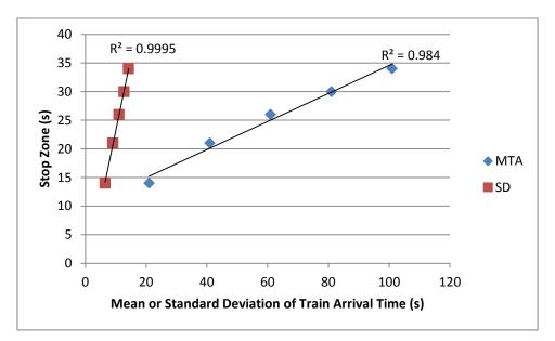
Figure 14. The Stop Zone as a function of the mean and standard deviation for  $\chi^2$  distributions.
