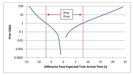
Figure 12. Prior odds as a function of difference from expected train arrival time. The  $\chi^2$  probabilities in Figure 10 were used to calculate the prior odds. The Stop Zone indicates the time during which motorists are likely to stop.
