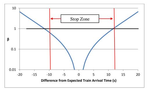
Figure 3. β as a function of difference from expected train arrival time. The Stop Zone indicates the time interval during which motorists are likely to stop.
