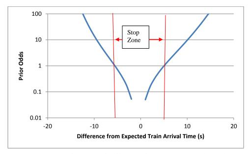
Figure 17. Prior odds as a function of difference from expected train arrival time. The Poisson probabilities in Figure 16 were used to calculate the prior odds. The Stop Zone indicates the time during which motorists are likely to stop.
