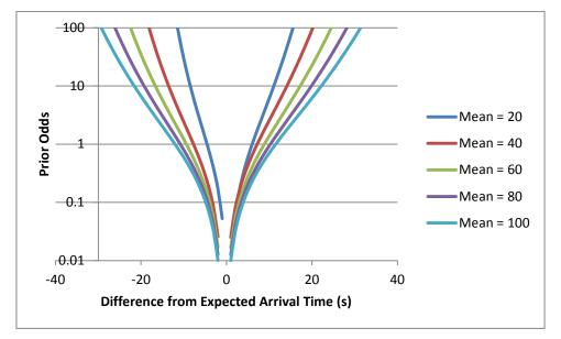
Figure 18. Prior odds as a function of the mean  $(\lambda)$  of the Poisson distribution.
