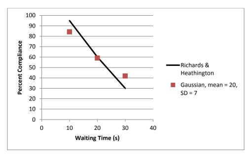
Figure 10. Percent motorist compliance as a function of waiting time. The data of Richards and Heathington are modeled by a Gaussian function.
