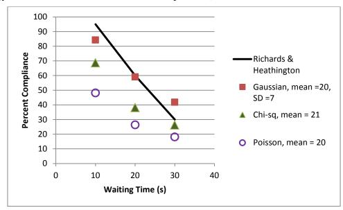
Figure 20. Percent motorist compliance as a function of waiting time for the Poisson,  $\chi^2$  and Gaussian models compared with empirical data from Richards and Heathington.
