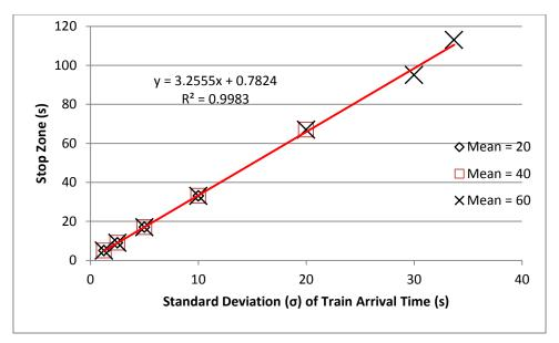
Figure 5. The Stop Zone width as a function of MTA and  $\sigma$ .
