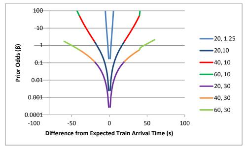
Figure 4. Prior odds as a function of  $\mu$  and  $\sigma$ .  $\mu$ s of 20, 40 and 60 s are shown with  $\sigma$ s of 1.25, 10 and 30 s.
