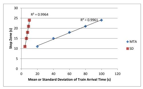
Figure 19. The Stop Zone as a function of the mean and standard deviation for Poisson distributions.
