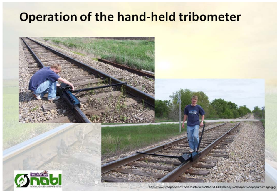
Figure 17: Tribometer measurements taken at mile intervals on both sides of the track
