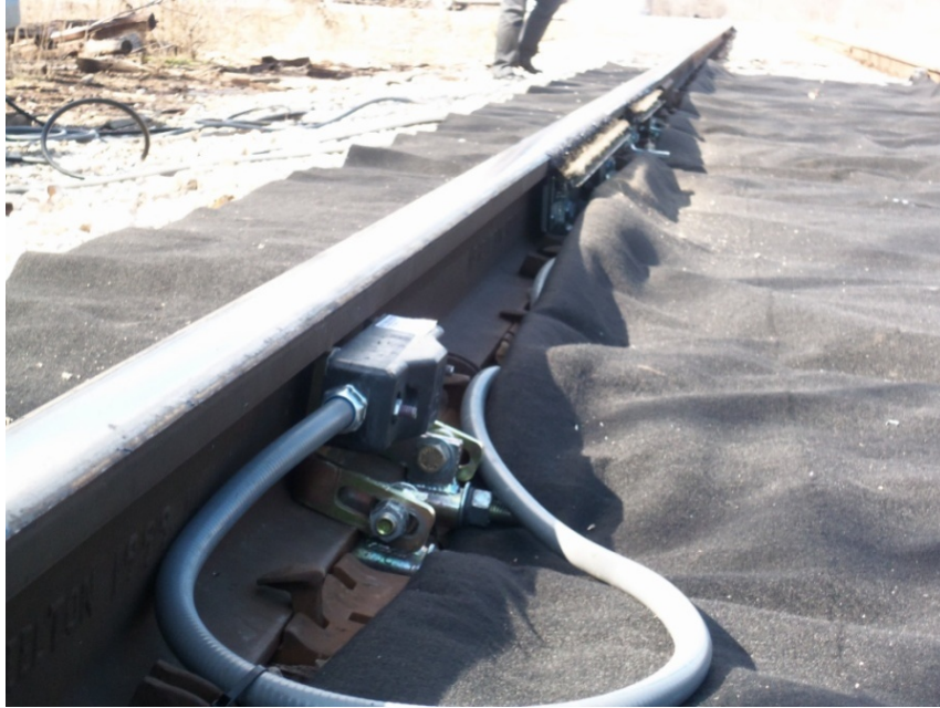
Figure 16: Track mats were used to collect any excess mineral oil-based grease at the lubricator site
