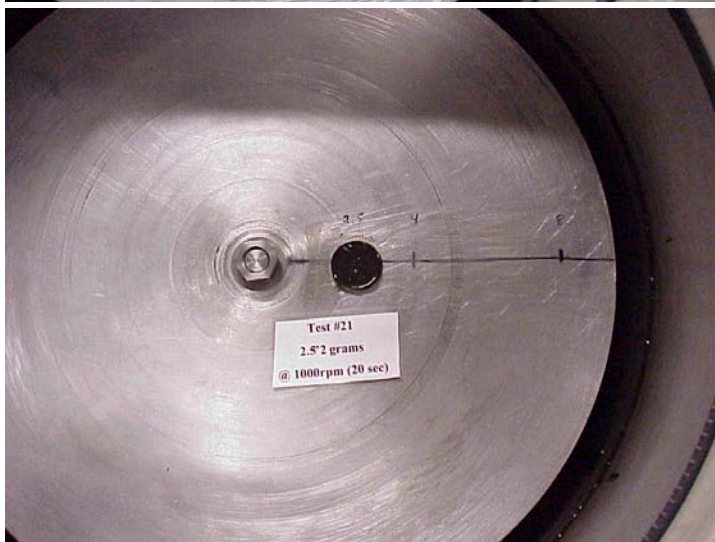
Figure 37: Patterns of the summer mineral oil-based grease #2 for 10 seconds and 20 seconds at 2½” distance from the disk center
