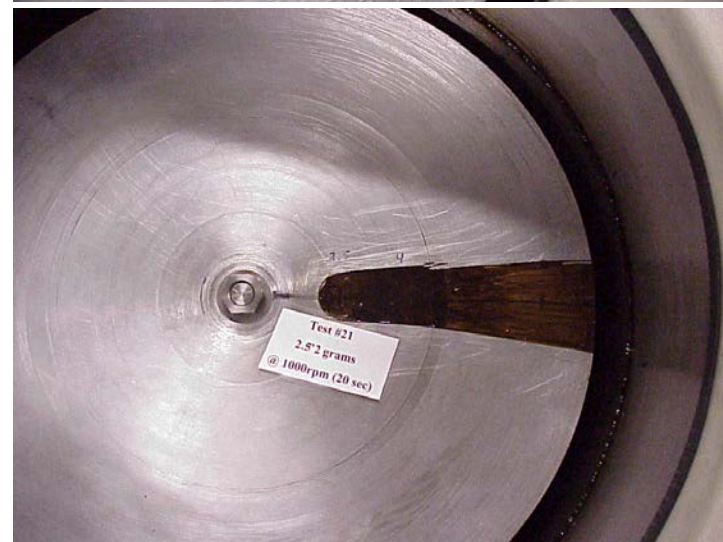
Figure 37: Patterns of the summer mineral oil-based grease #2 for 10 seconds and 20 seconds at 2½” distance from the disk center
