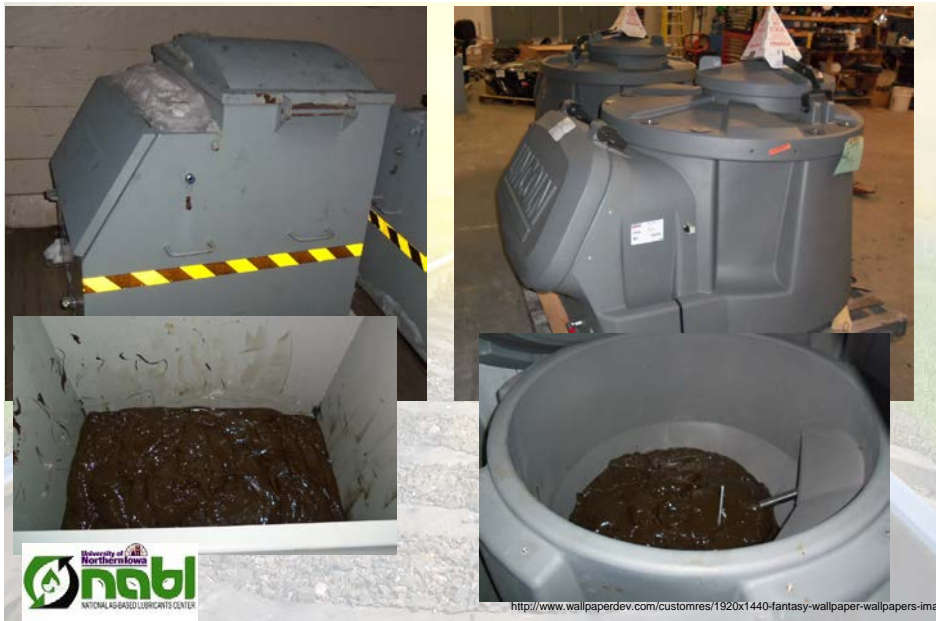
Figure 3: The test grease dispensers from two OEMs
