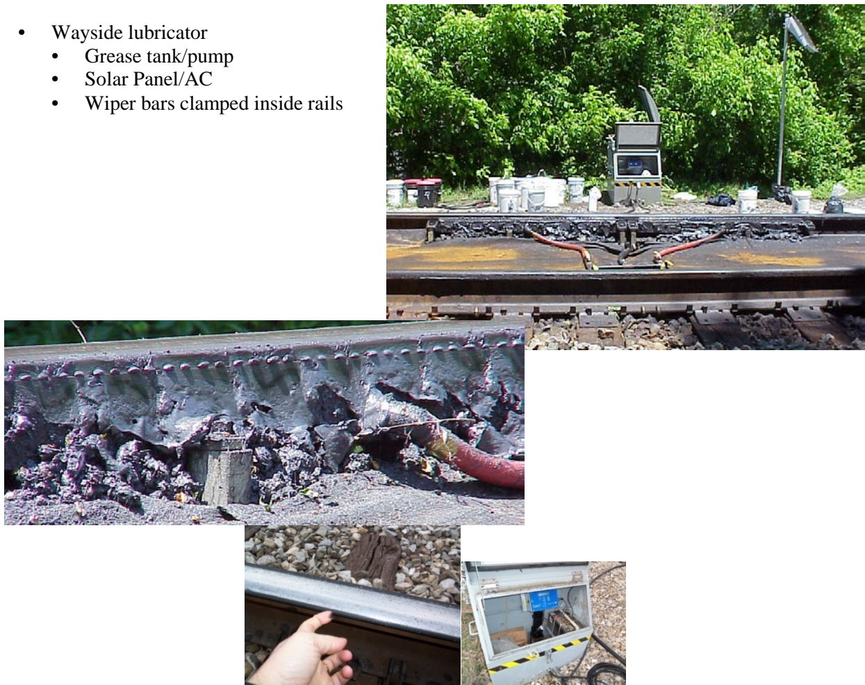
Figure 1: Basic components of a wayside grease dispenser (lubricator) and grease on gage face
