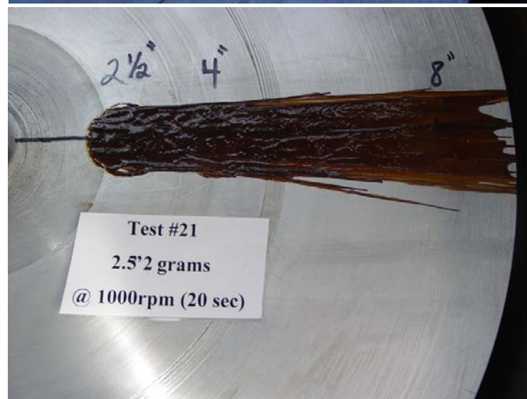
Figure 31: Patterns of the winter bio-based grease #2 for 10 seconds and 20 seconds at 2½" distance from the disk center
