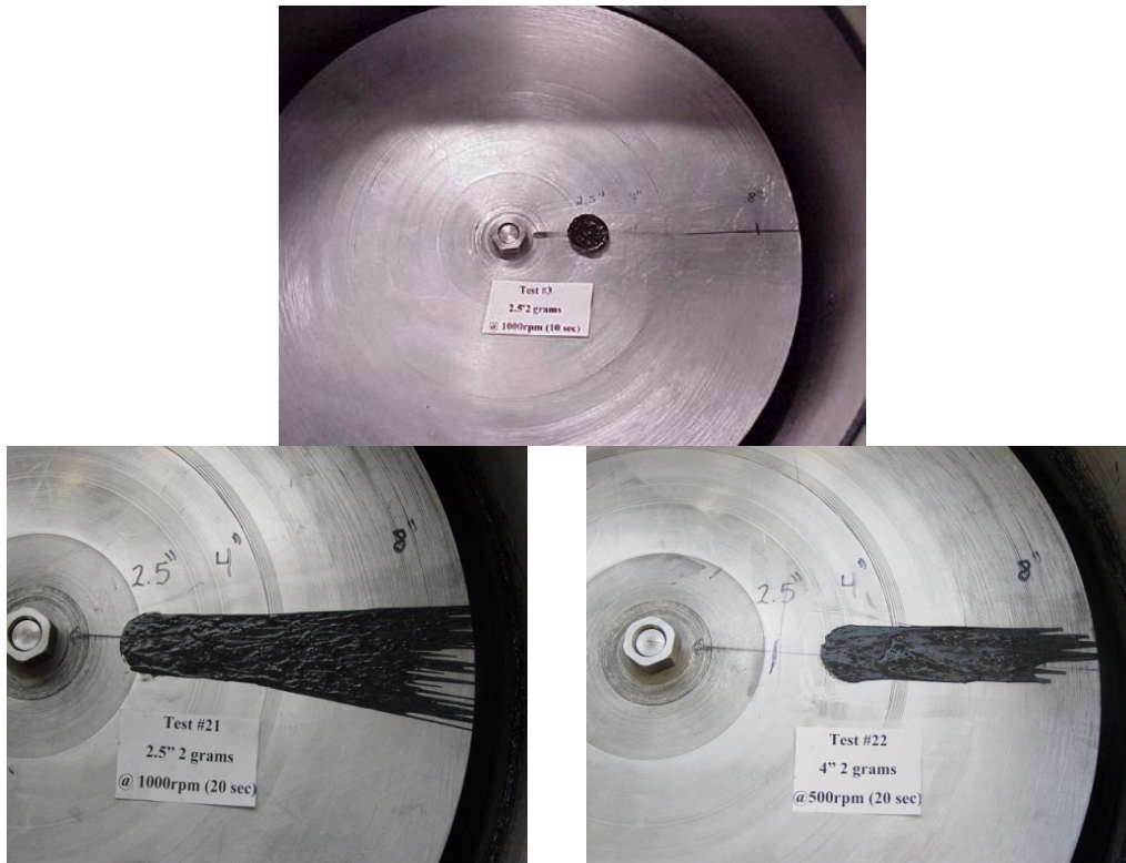
Figure 28: An aluminum disk with 18” diameter inside a centrifuge for testing grease tackiness
