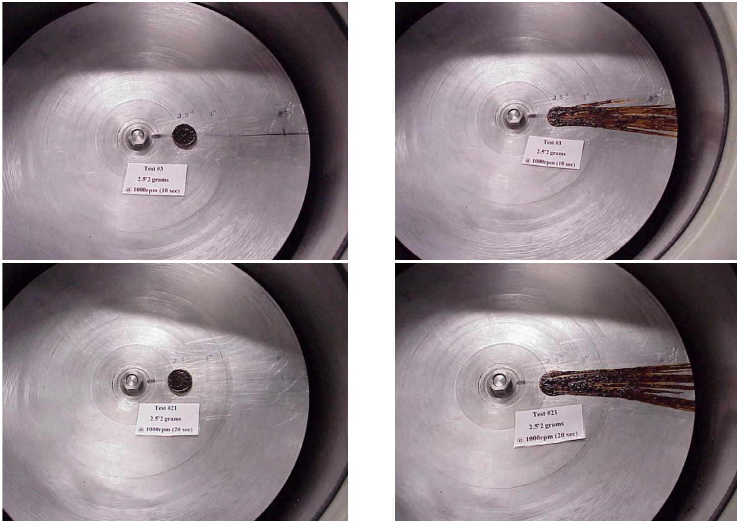
Figure 34: Patterns of the summer bio-based grease #2 for 10 seconds and 20 seconds at 2½” distance from the disk center
