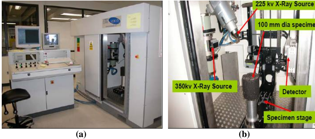
Figure 16 - a) Overall X-ray CT System and Shielding Cabinet; b) Mini- and Micro-focus System
