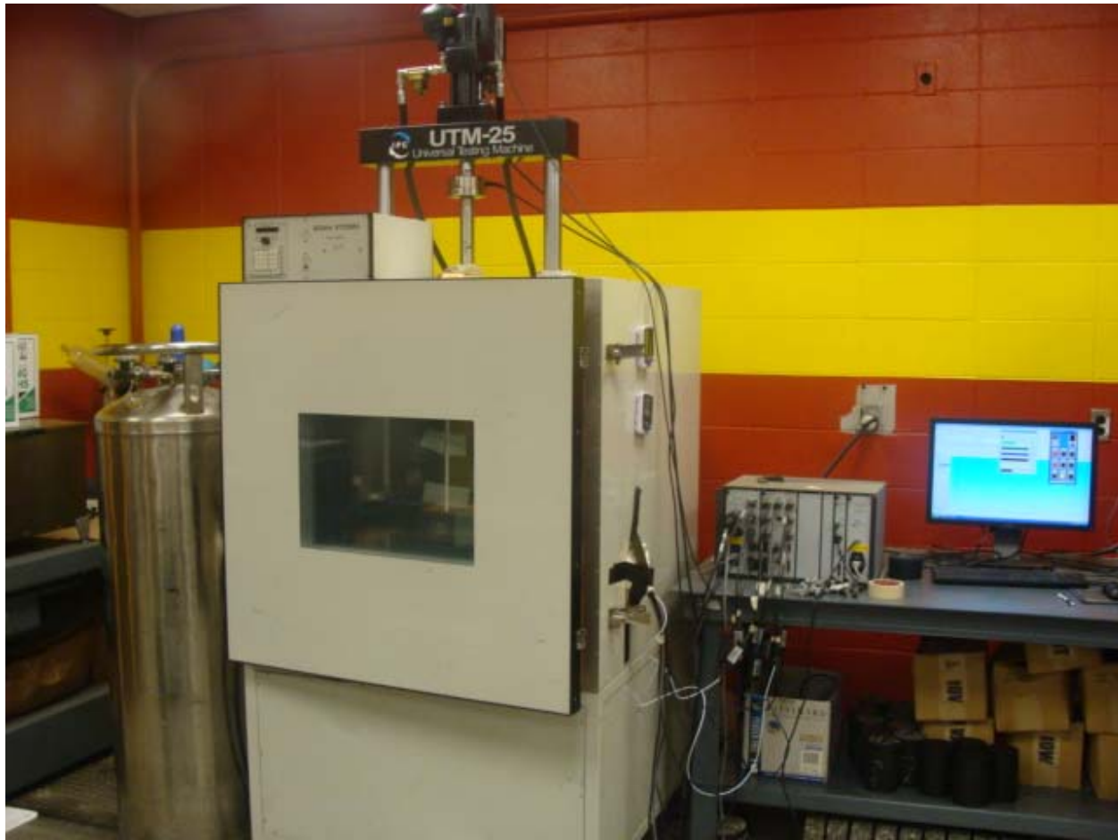
Figure 4.11: UTM-25 Machine for Dynamic Modulus Testing
