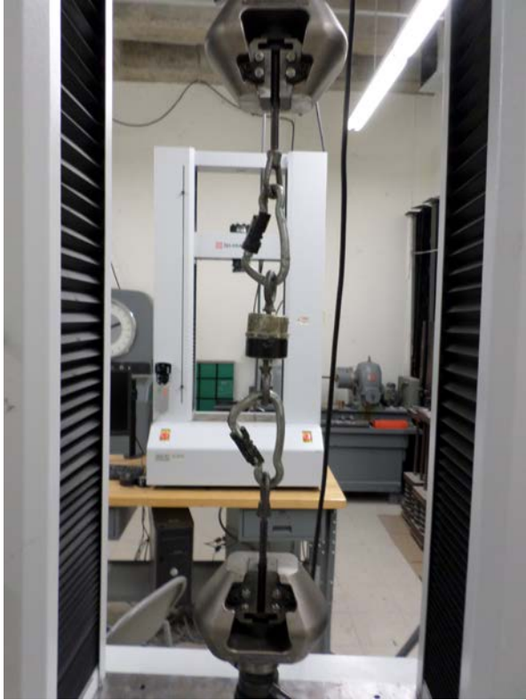
Figure 6.9: Epoxy Tensile Test Setup
