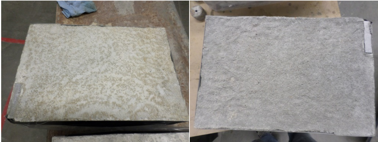
Figure 4.12: Before (left) and After (right) Sandblasting a Slab
