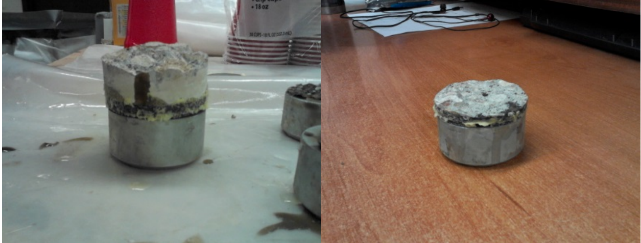
Figure 4.26: Failure Type 1 (left) and Failure Type 2 (right)
