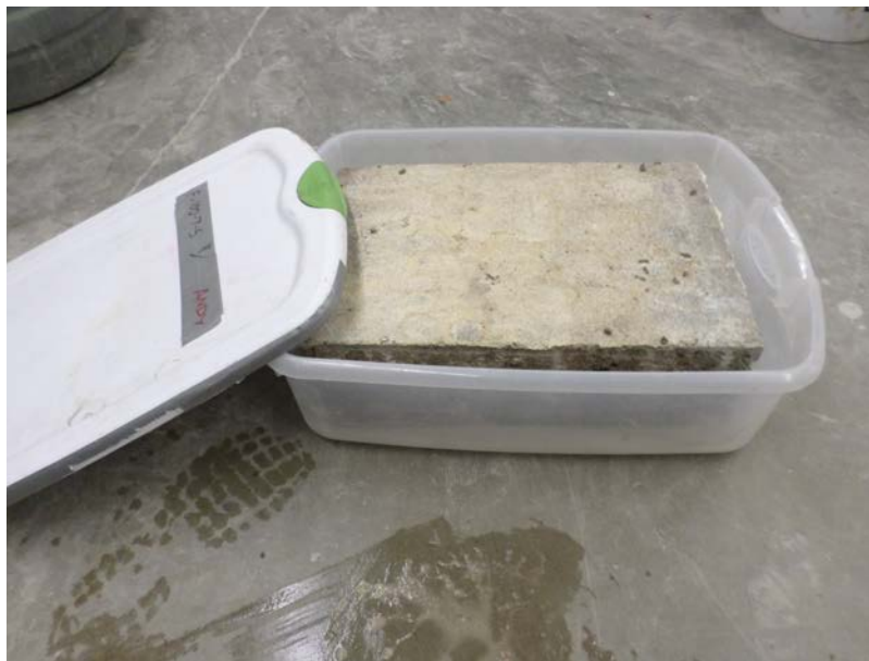
Figure 4.7: Slab Placed Inside a Bin for Wet Curing
