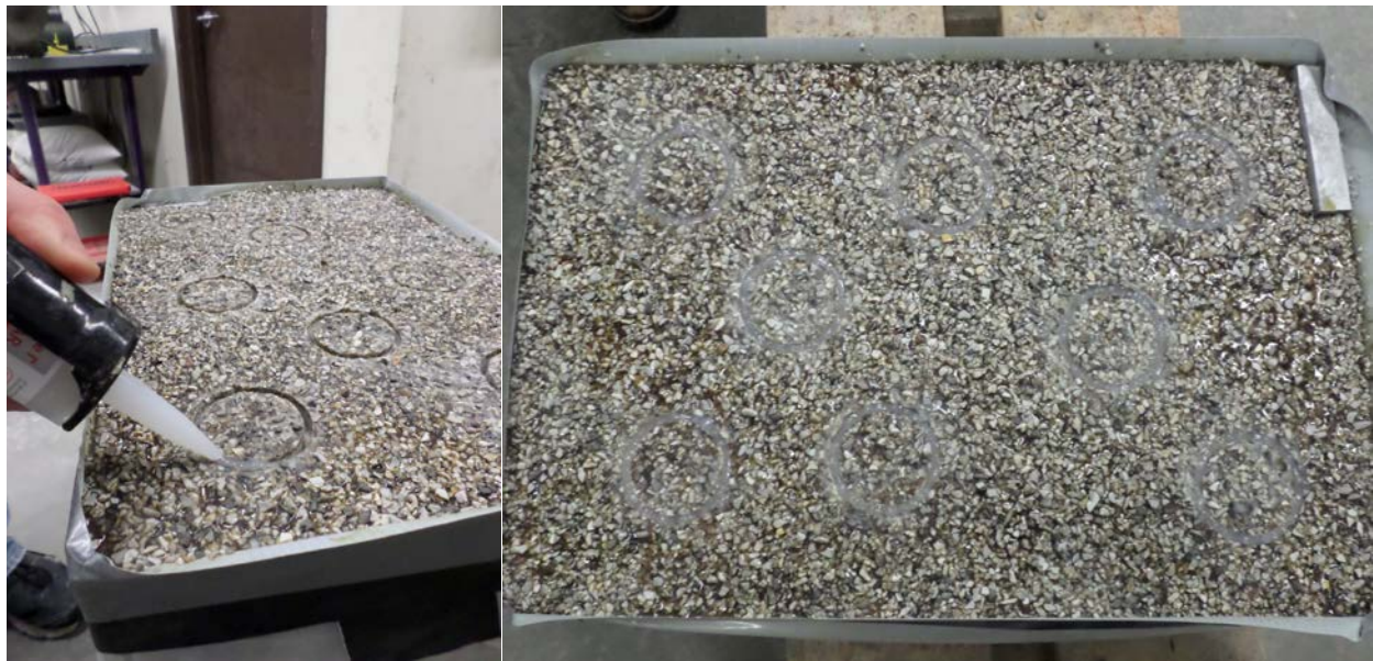
Figure 4.19: Placement of Silicone Caulk to Seal the Cores
