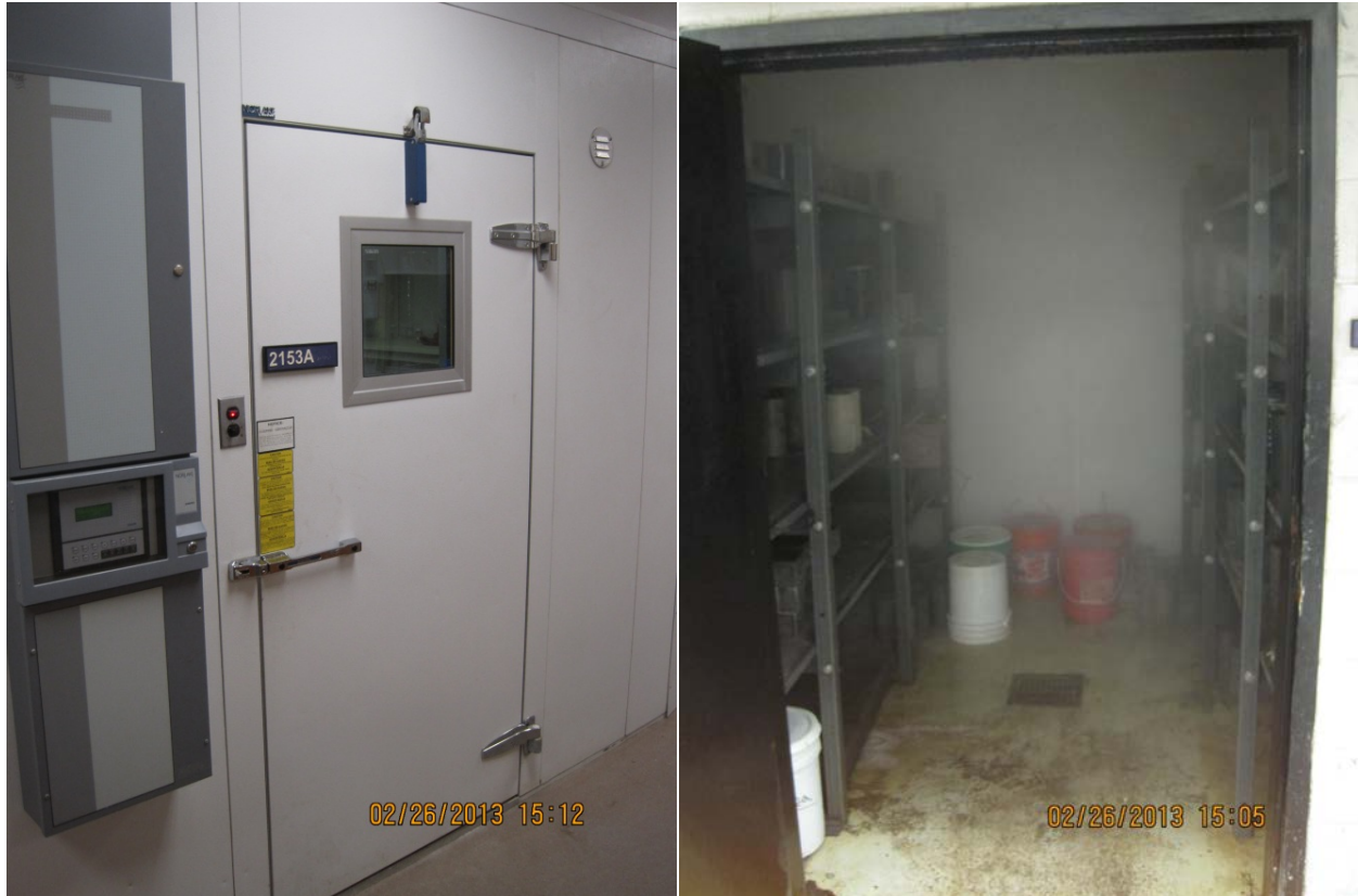
Figure 4.5: Wet Cure Locations for 40°F Refrigerator (left) and 73°F Moist Room (right)
