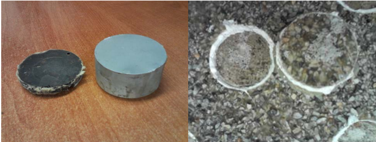
Figure 4.28: Failure Type 5 (left) and a Failure with Both Type 2 and Type 3 (right)
