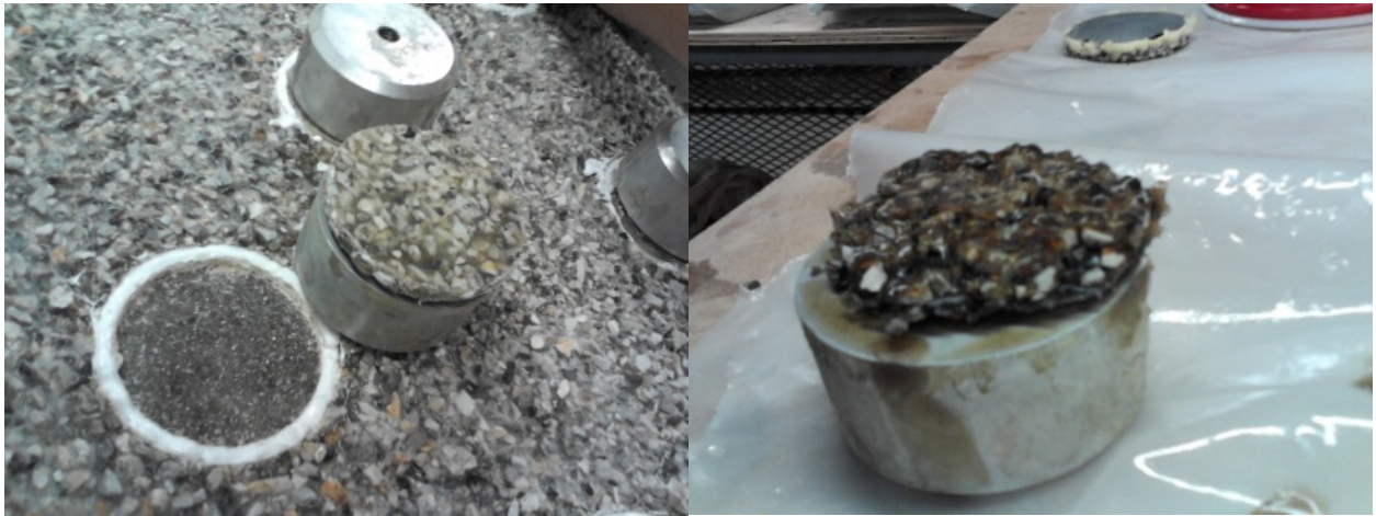
Figure 4.27: Failure Type 3 (left) and Failure Type 4 (right)
