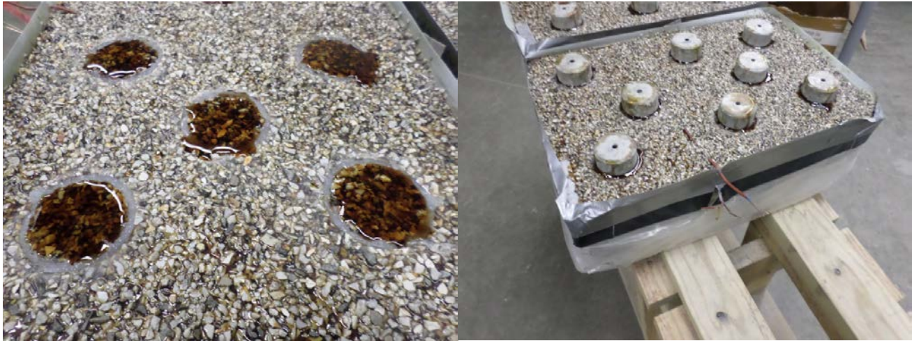
Figure 4.21: Slabs Before and After Placing Pull-Off Caps
