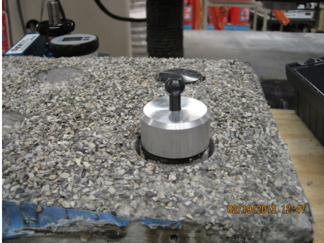
Figure 4.25: Pull-Off Cap Ready to be Tested
