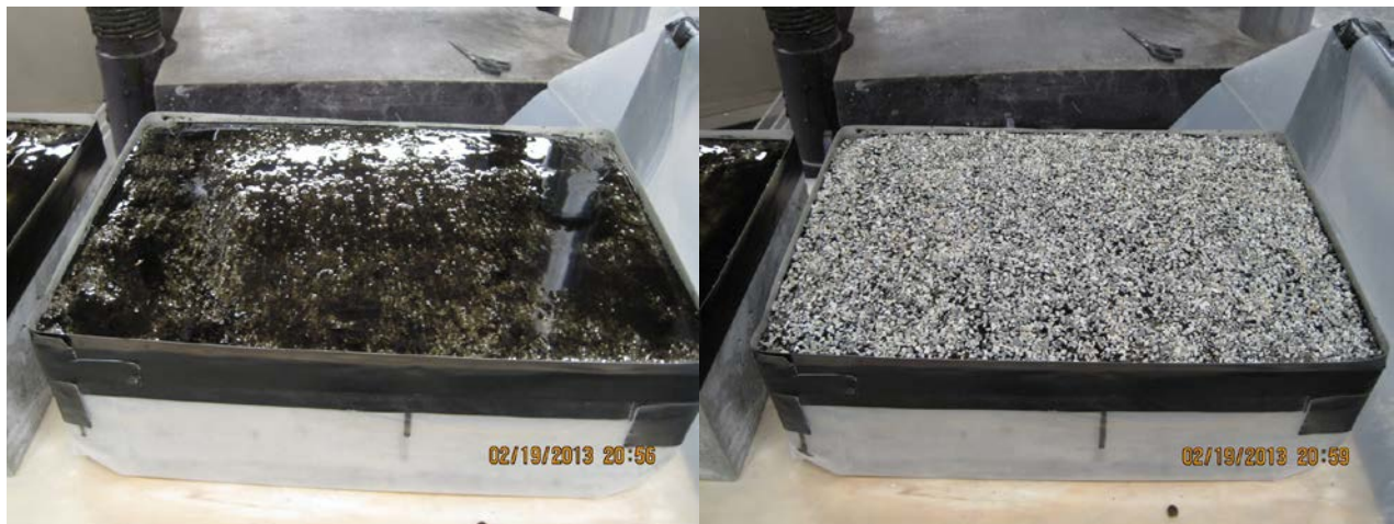
Figure 4.16: Placement of Course One of Epoxy (left) and Aggregate (right)
