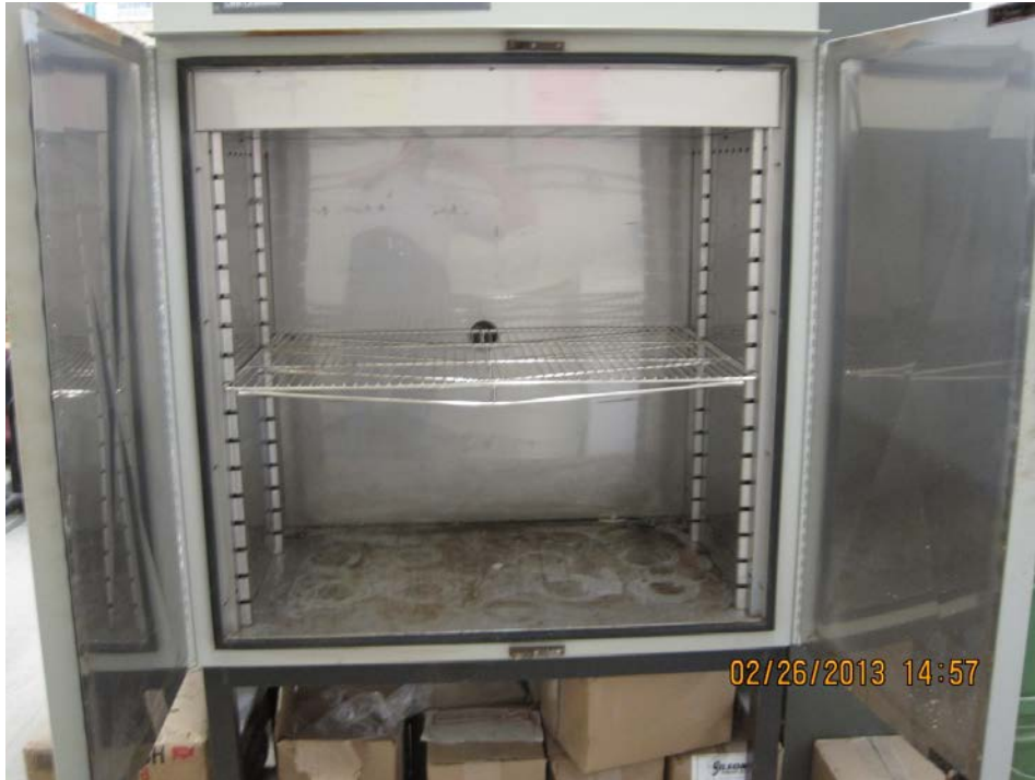
Figure 4.6: Wet Cure Location for 100°F Oven
