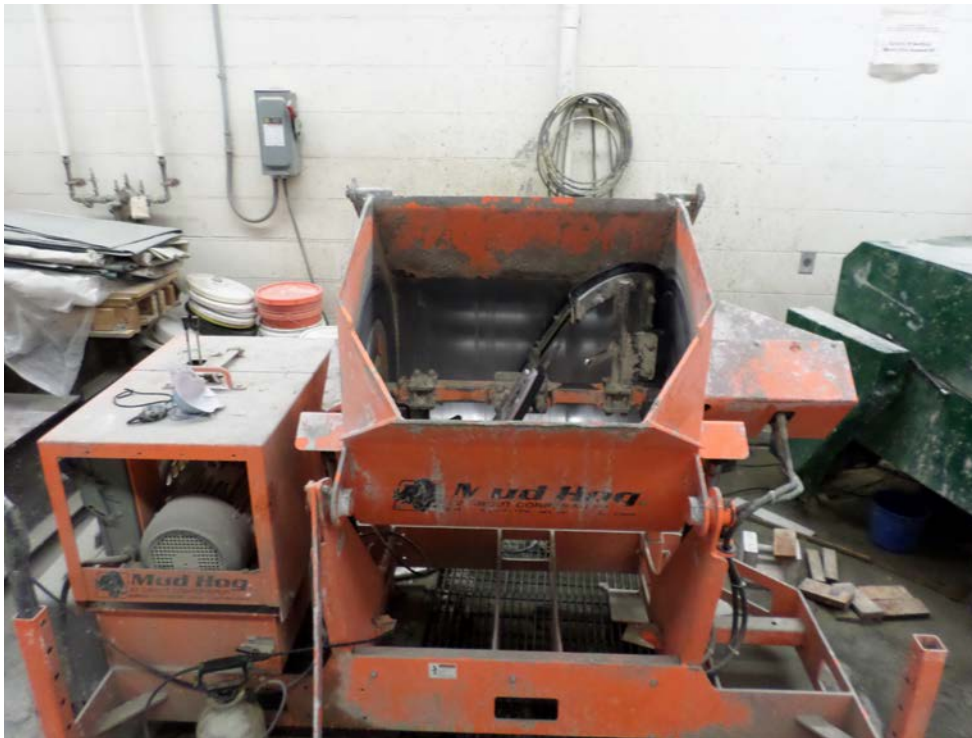
Figure 4.3: Mud Hog Mixer Used to Batch Concrete
