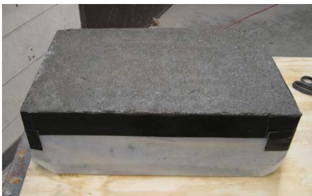
Figure 4.9: Slab Wrapped in Plastic to Dry
