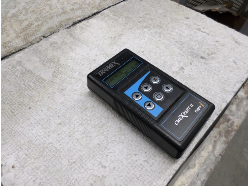
Figure 4.15: Tramex CMEXpert II Instrument Used to Take Moisture Readings
