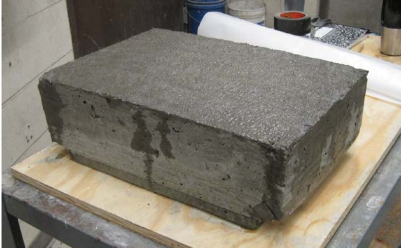
Figure 3.3: Slab after Wet Curing
