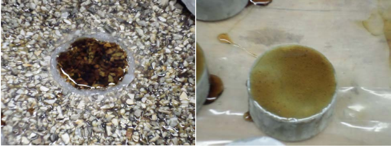
Figure 4.20: Application of Adhesive Epoxy to Mount the Aluminum Caps
