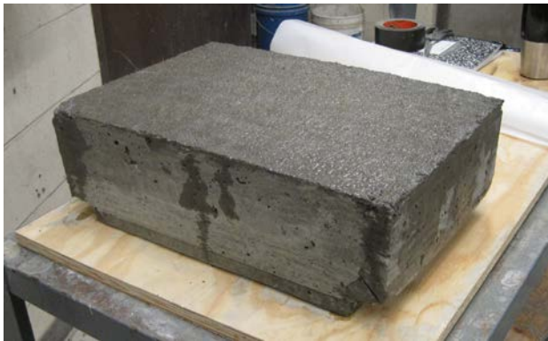
Figure 4.8: Slab After Wet Curing
