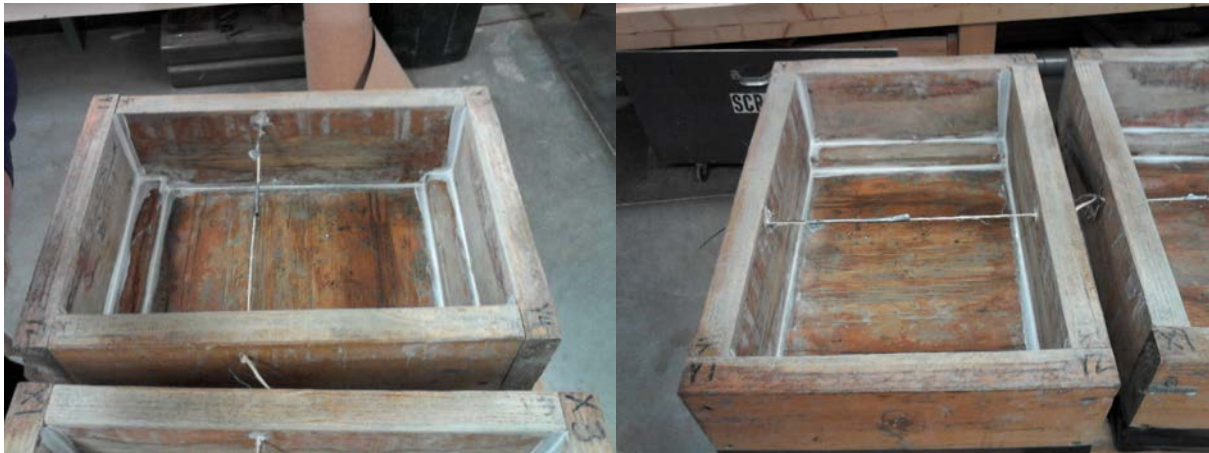
Figure 4.1: Forms Built to Accommodate the 12×18×6-Inch Slabs
