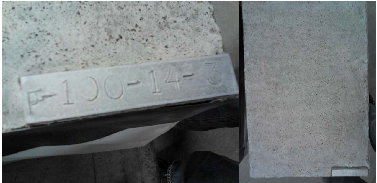
Figure 4.4: Slab Label Cast into the Concrete
