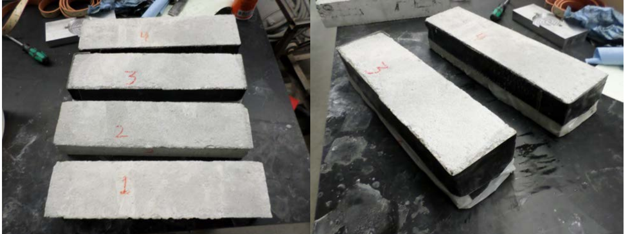
Figure 6.2: Test Specimen Cast to Test Moisture Content
