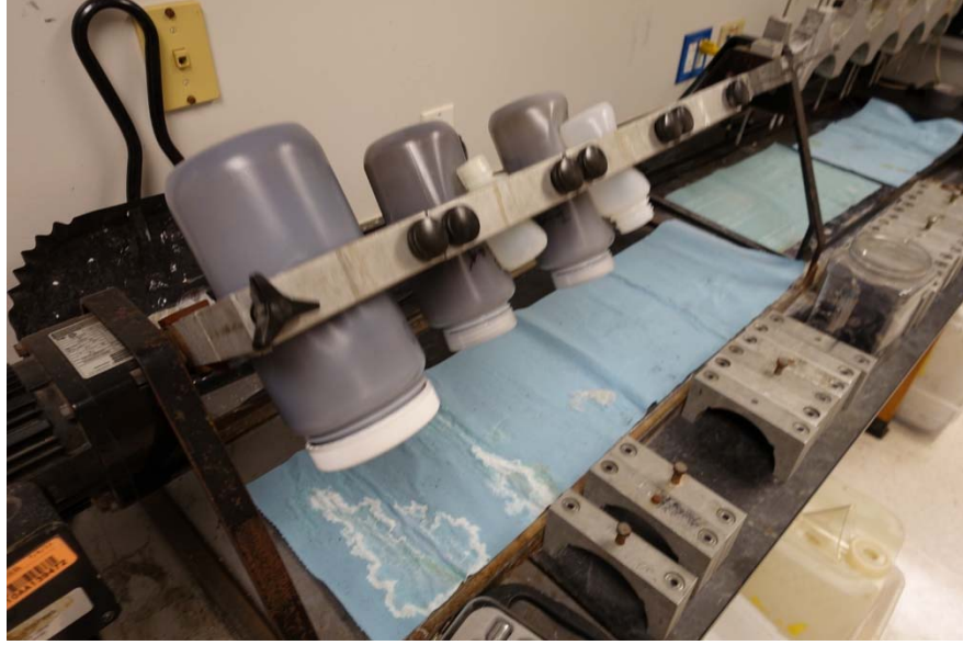
Figure 5. Mixing FA and ammonium sulfate salt on a rotator to create spiked FA samples.
