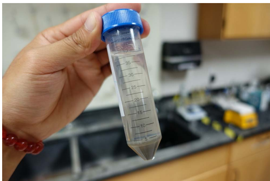
Figure 15. Extraction using a 50-mL centrifuge tube.
