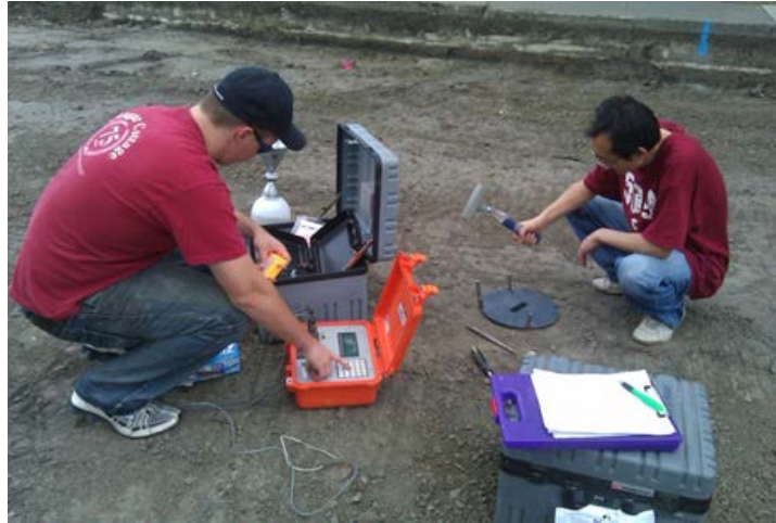
Figure 6. Team Members Setting Up the Electrical Density Gauge C Model
