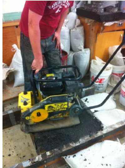
Figure 14. Laboratory Compaction Using Vibratory Plate Compactor
