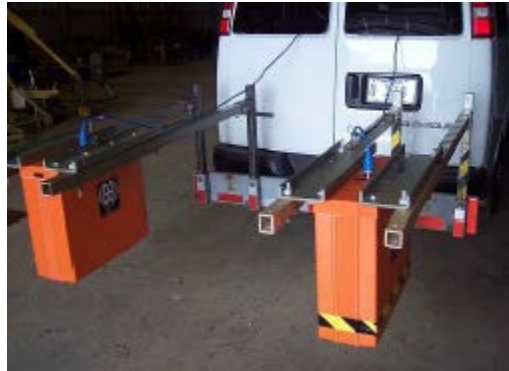
Figure 5. Air Coupled GPR System (16)
