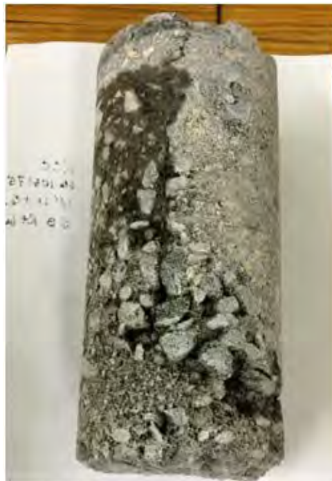
Figure 18. Core Through Stop-and-Go Section
