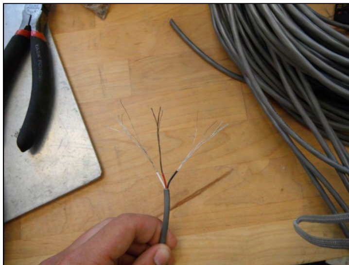
Figure A-2. Stripped 22 AWG Wire
