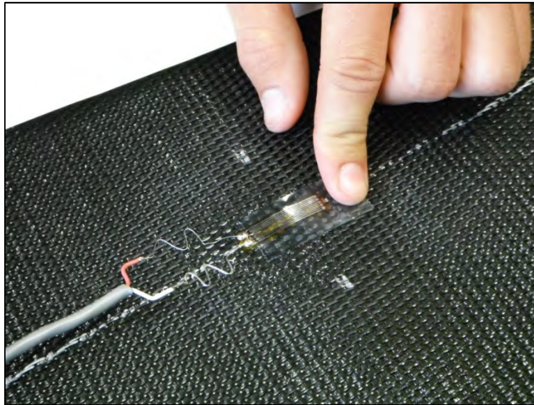
Figure A-8. Positioning the Strain Gage on the Geotextile
