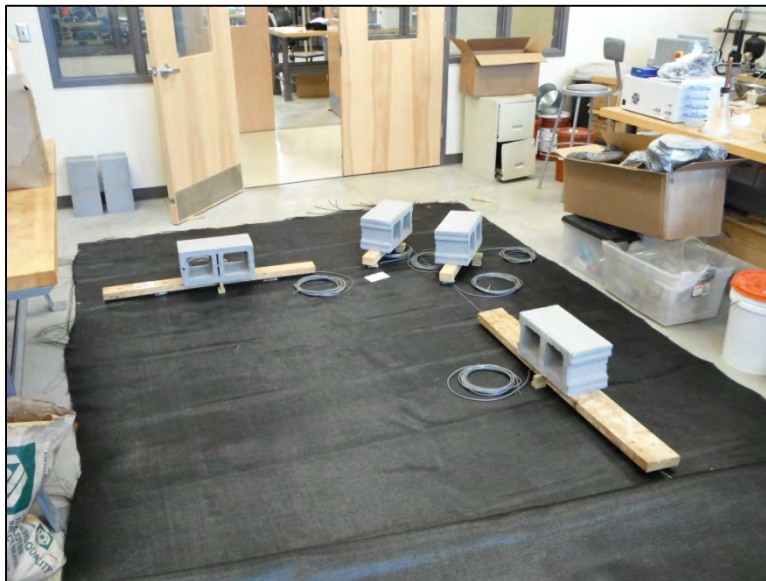
Figure A-13. Spacing and Configuration of 8 Strain Gages Installed at One Time
