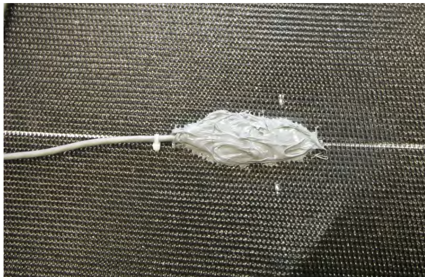
Figure A-15. Finished Strain Gage Protected by RTV
