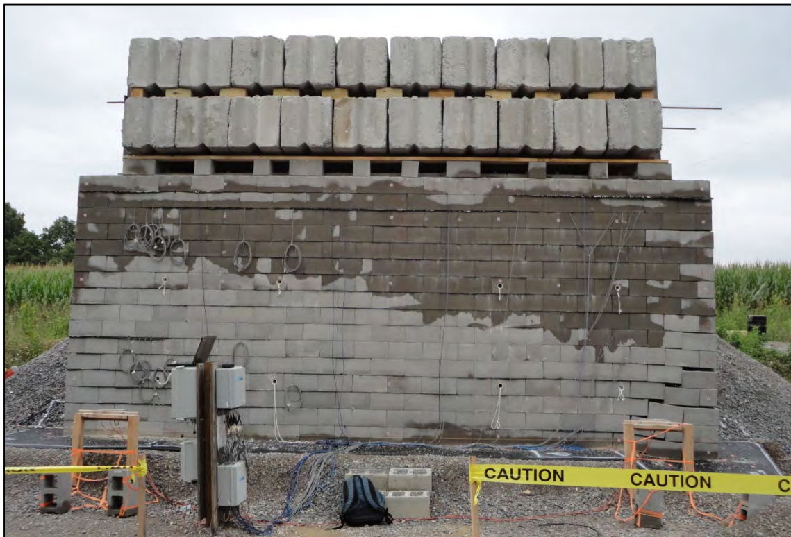
Figure 26. Front View of Abutment After Test A1
