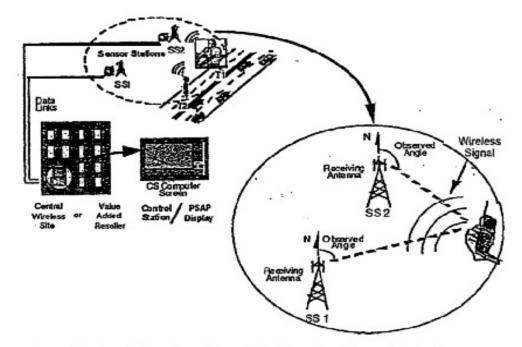
Determination of Location with Multiple Sire LOB "Cross-Fixing" System
