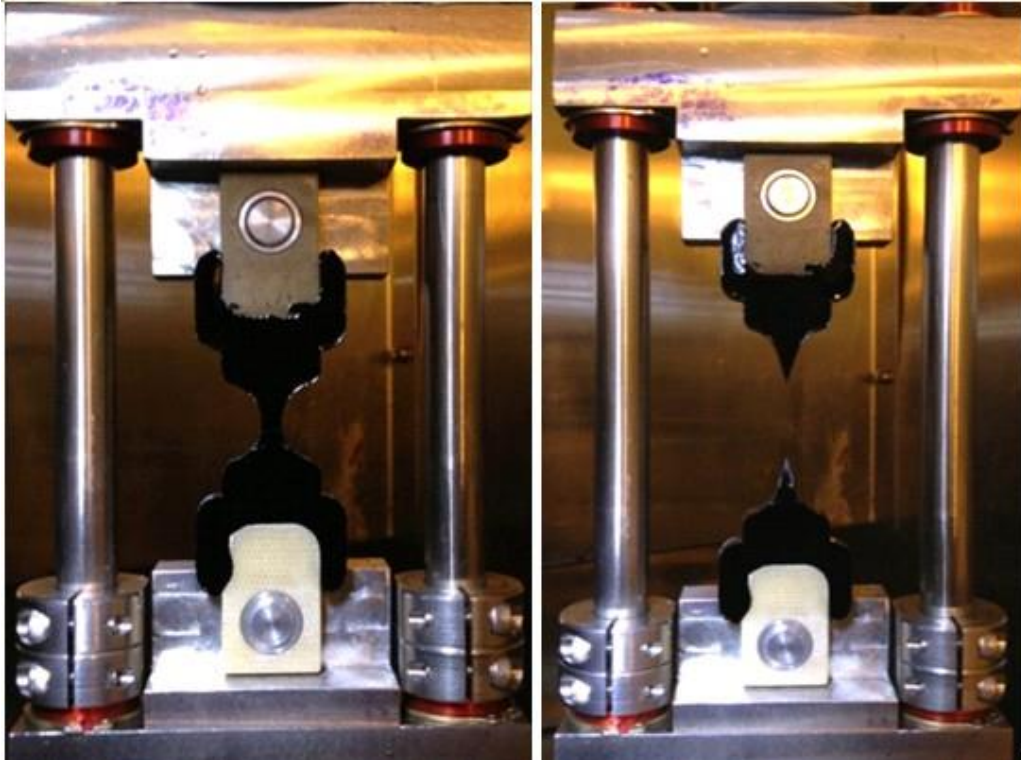
Figure 3-10 Specimen configurations before (A) and after (B) BFE test (Yan et al, 2015)
