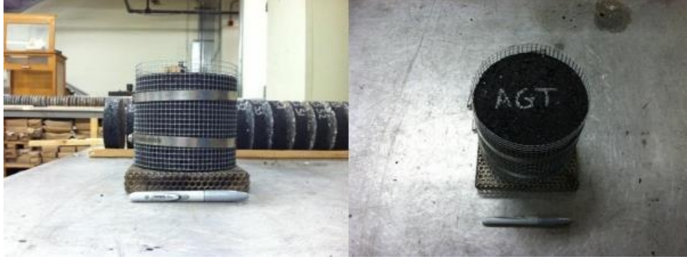
Figure 3-17 Specimens setup for LTOA conditioning
