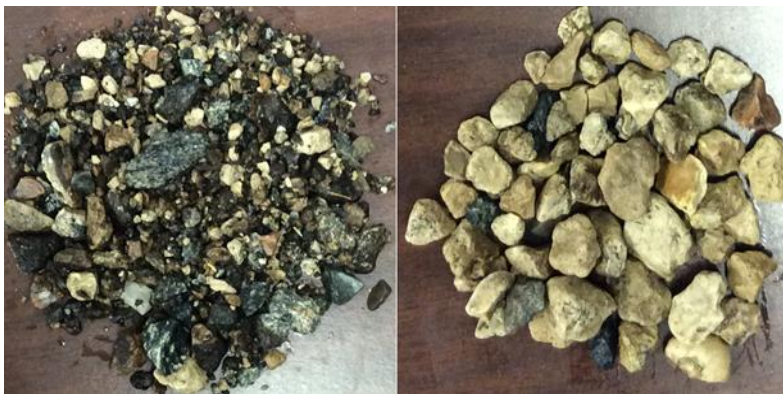
Figure 3-2 Aggregate components of ATL (left) and WH (right) RAP
