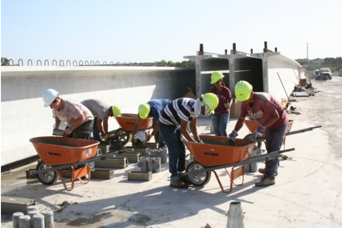
Figure B.30. Test Specimen Casting.
