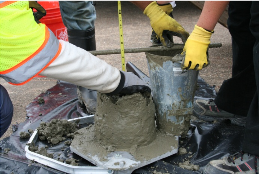
Figure B.28. Slump Measurement (CC).
