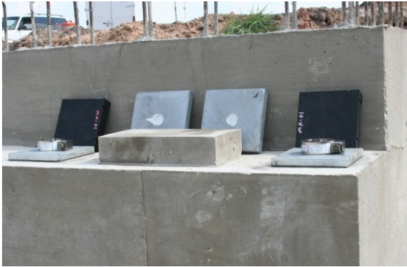
(a) South End Load Cell Assembly and Layout
