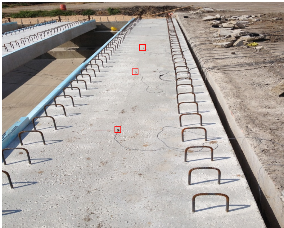
Figure 4.7. Accelerometer Positions for Individual Beam Test.
