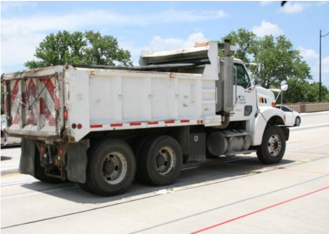
(b) Static Load Test with TxDOT Dump Truck
