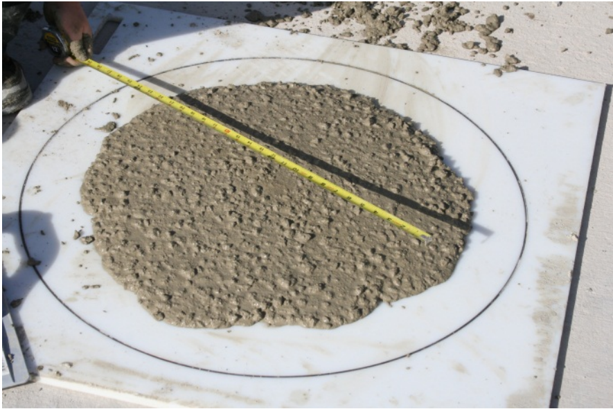
Figure B.29. Slump Measurement (SCC).
