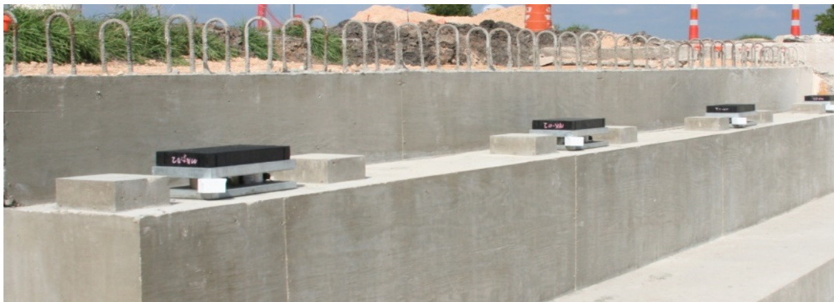
(b) North End Load Cell Layout
