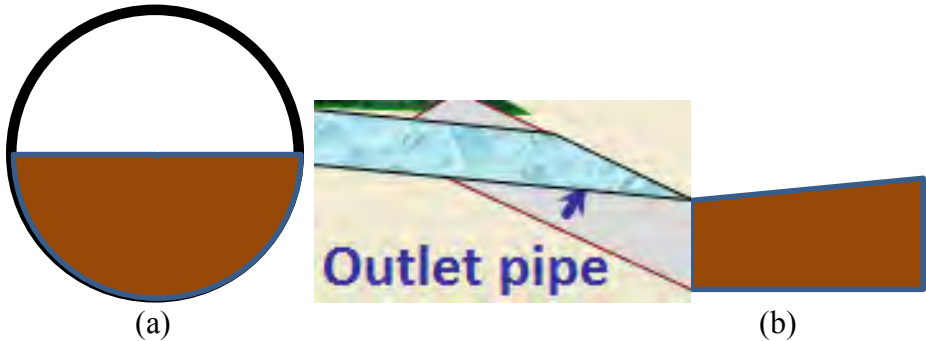
Figure 7. Subdrain outlet functional rating based on visual observation: (a) 50 percent blockage, and (b) up-hill condition of surface at the outlet end
