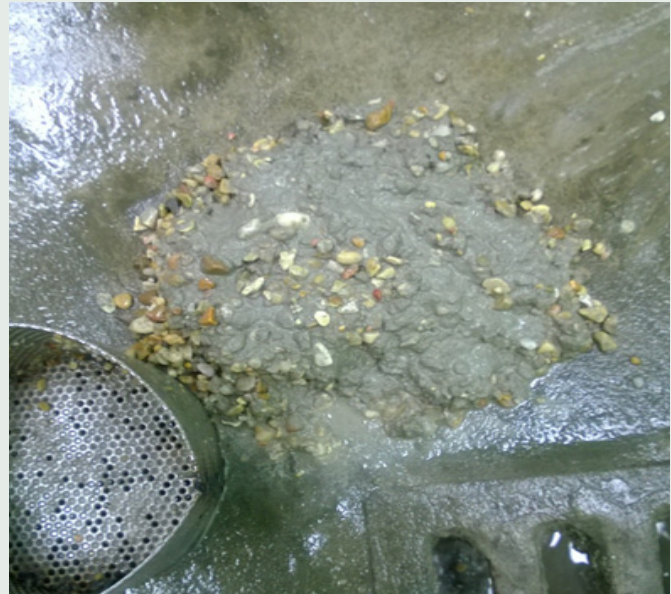
Figure 2 Washout test result for a No. 8 pea gravel mixture incorporating a VMA showing cement paste
