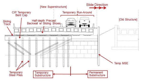
Figure 1–11 Section through the deck of the new superstructure (at abutment) on temporary location
