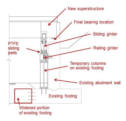
Figure 1–2 Section through an existing abutment with sliding accessories
