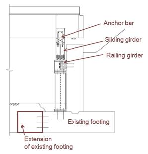
Figure 2–5 Section through dependent backwall
