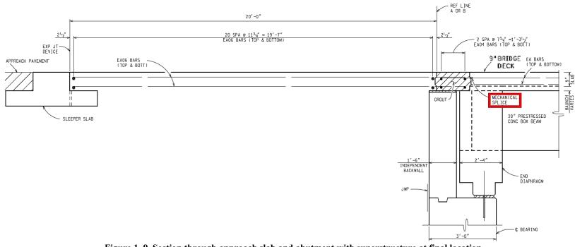
Figure 1–9 Section through approach slab and abutment with superstructure at final location
