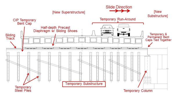
Figure 1–10 A section through the new superstructure deck (at pier) on temporary location
