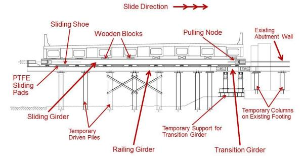
Figure 1–1 Section through the deck of the new superstructure on temporary structure
