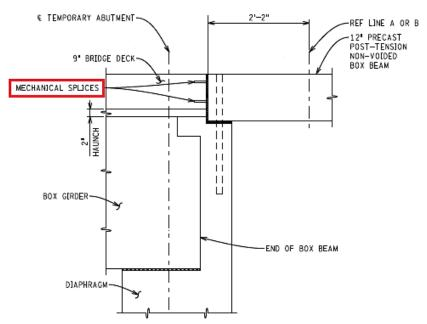
Figure 1–7 Section through the abutment with superstructure at temporary location
