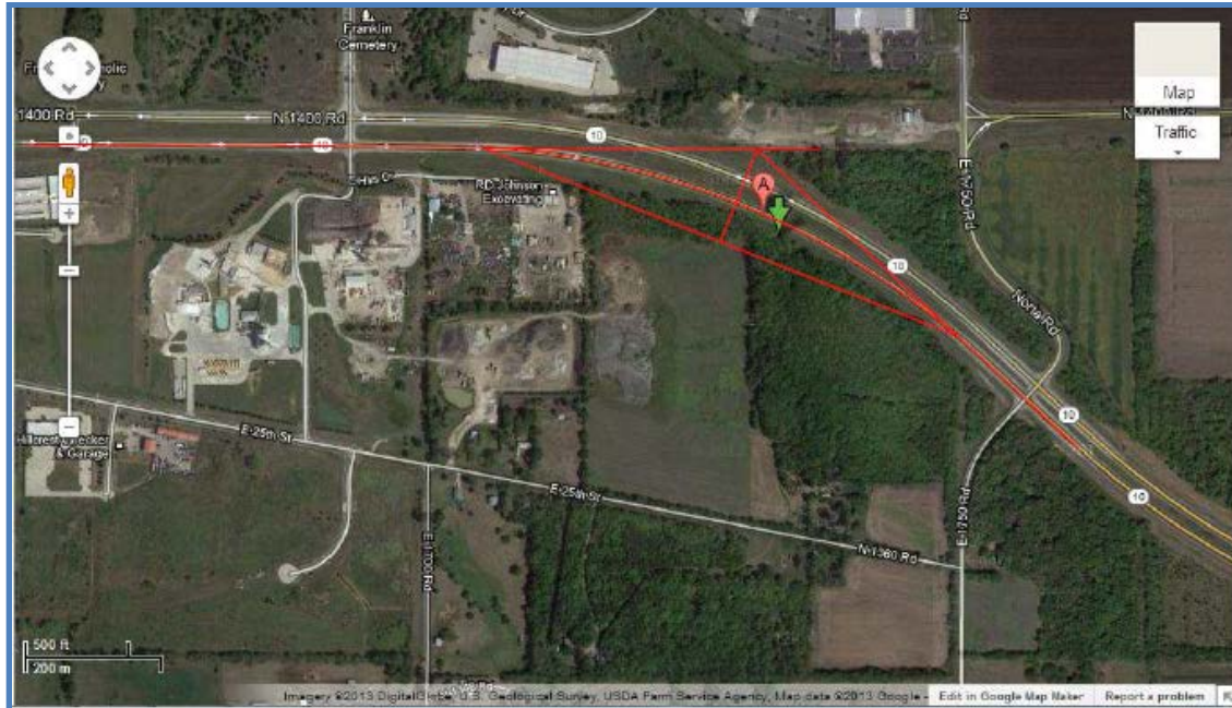
Figure 2.2: Determining Characteristics of a Curve Using Google Maps and AutoCAD Source: Google, n.d.
