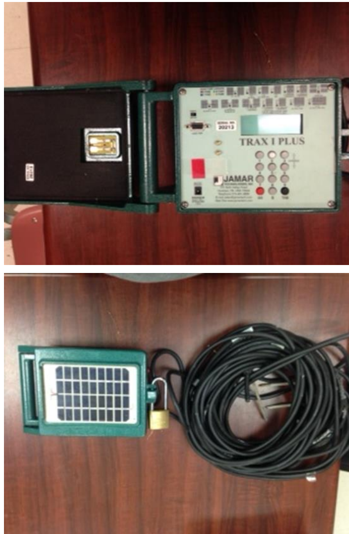
Figure 3.7. TRAX I Plus traffic counter photos
