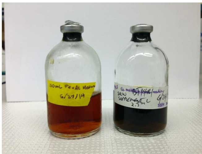
Figure B1. G. metallireducens grown in iron(III)-acetate medium, with iron(III) as the electron acceptor and acetate as the electron donor. When inoculated, the medium turned from amber to dark green as iron(III) was biologically reduced to iron(II).
