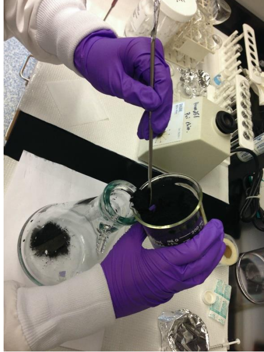
Figure D1. Sieved biochar, particle size range 0.25-0.50 mm.
