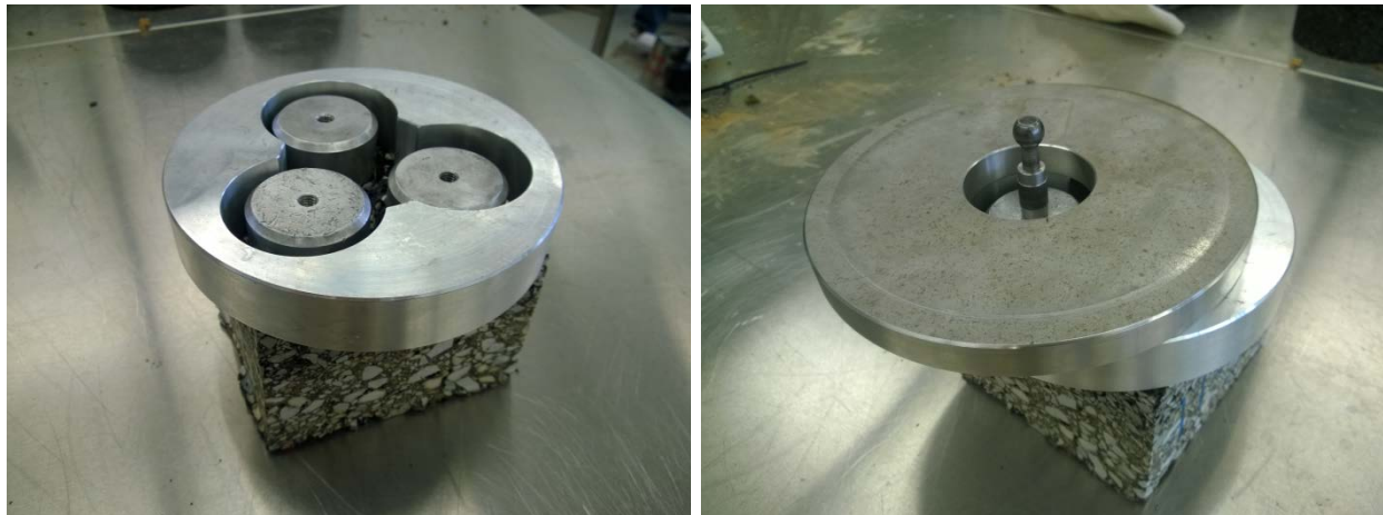
Figure 4. Prepared Sample with Reaction Plates.
