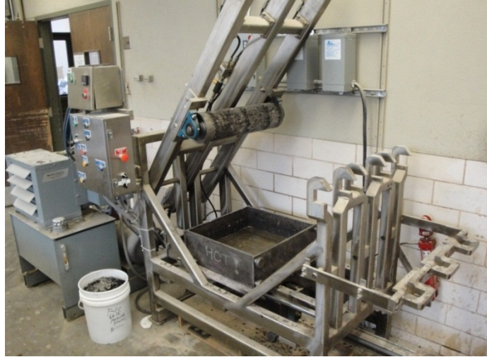
Figure 3.2. PMW Linear Compactor for Molding Slabs.
