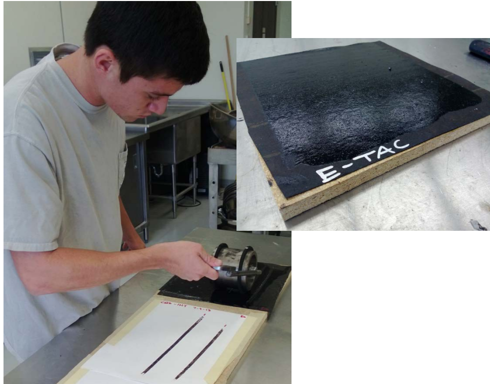
Figure 4.14. Tack Tracking BASF Roller Test.
