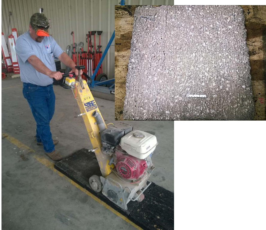
Figure 4.8. Applying Simulated Milled Texture.
