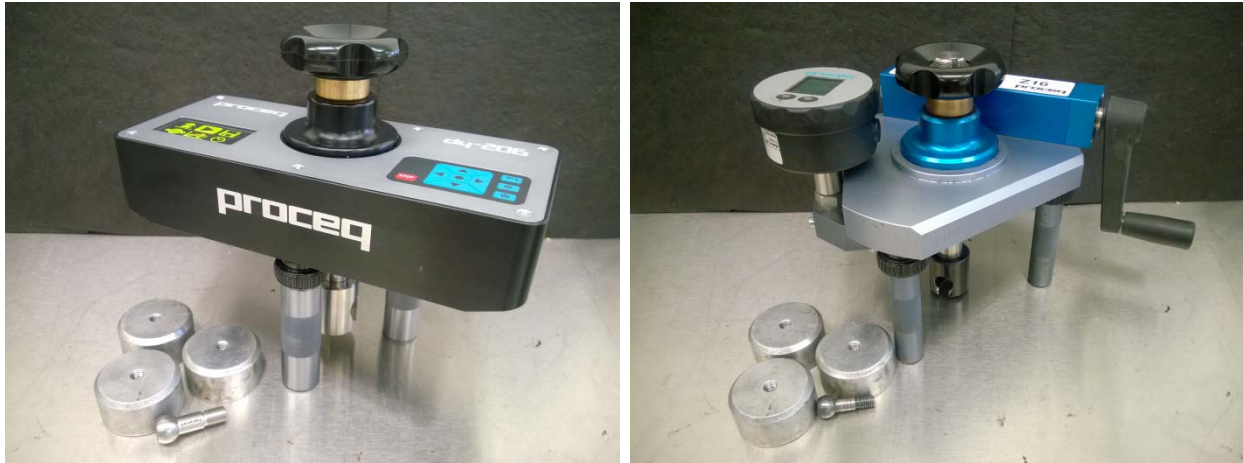
Figure 1. Proceq DY-2 (Left) and DynaZ (Right) Pull-Off Testers.
