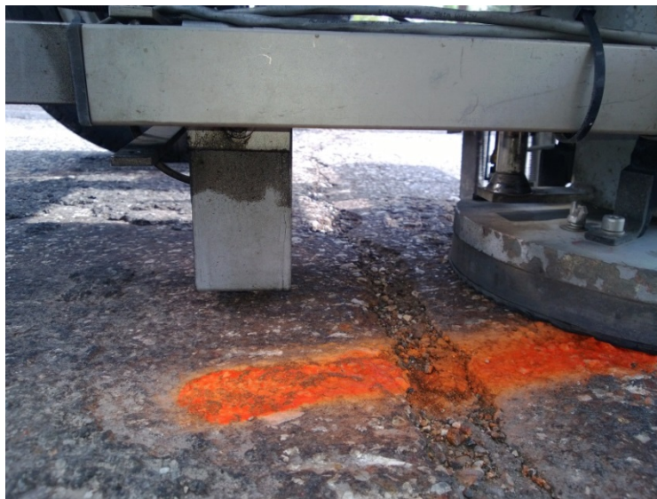
Figure 6.4. Load Transfer Testing with an FWD.
