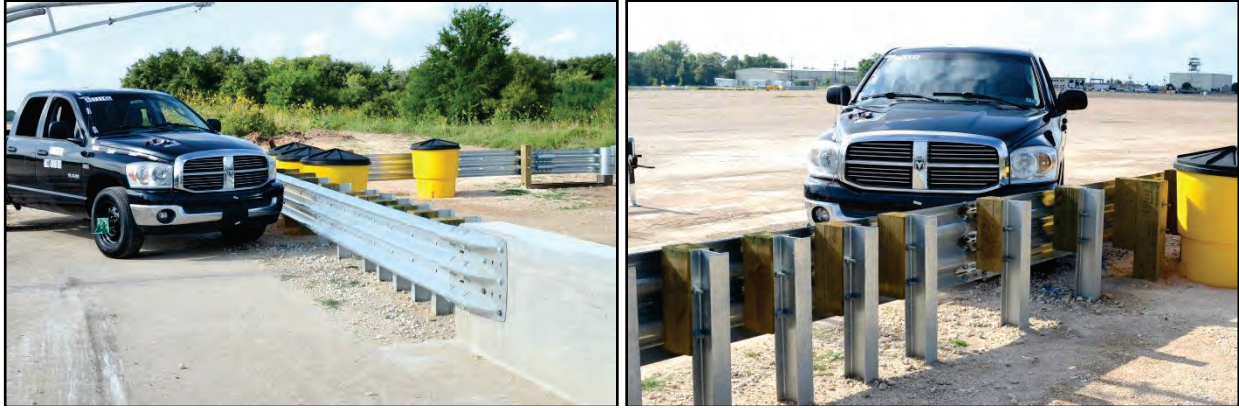
Figure 7.19. Vehicle/Installation Geometrics before Test No. 467114-6.
