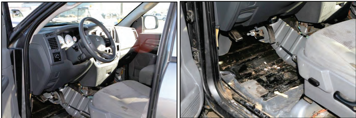
Figure 7.5. Interior of Vehicle after Test No. 467114-3.
