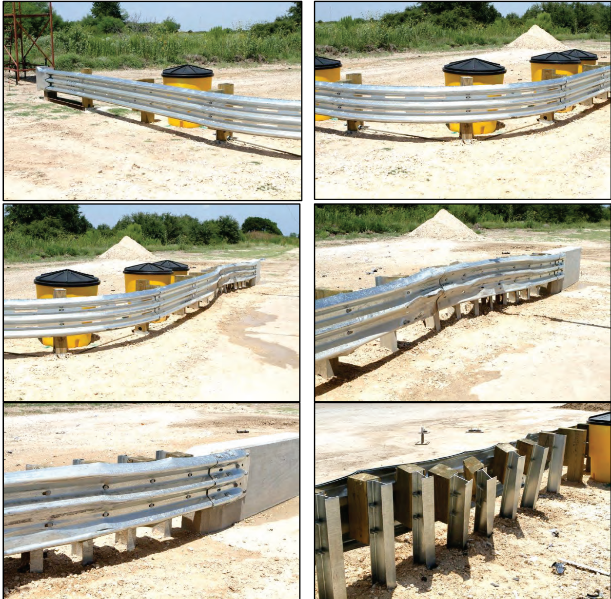
Figure 7.26. Installation after Test No. 467114-7.
