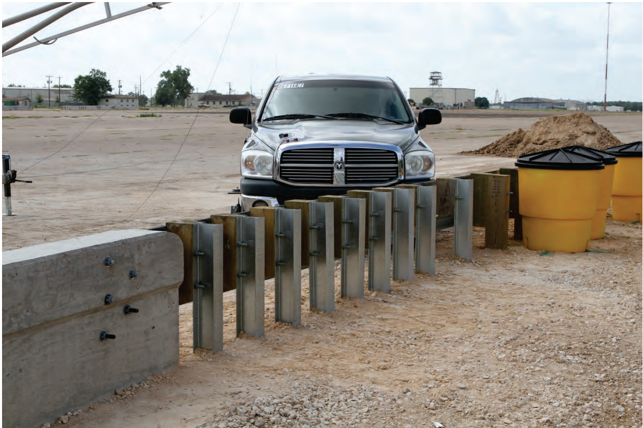
Figure 5.8. Short Radius Guardrail (Primary Road) before Test No. 467114-7.
