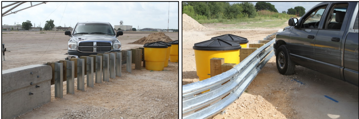
Figure 7.24. Vehicle/Installation Geometries for Test No. 467114-7.
