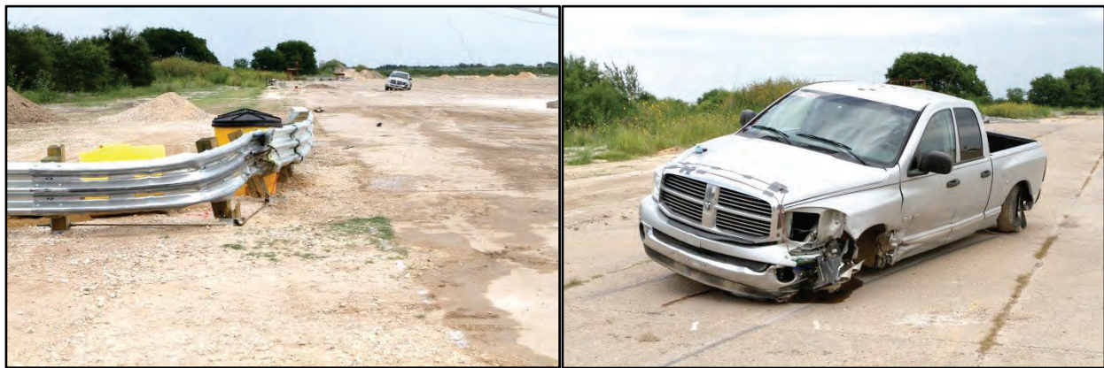
Figure 7.14. Vehicle/Installation after Test No. 467114-5.
