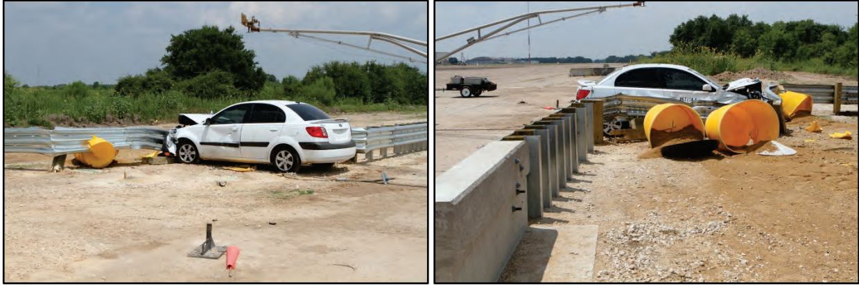
Figure 7.8. Vehicle/Installation after Test No. 467114-4.
