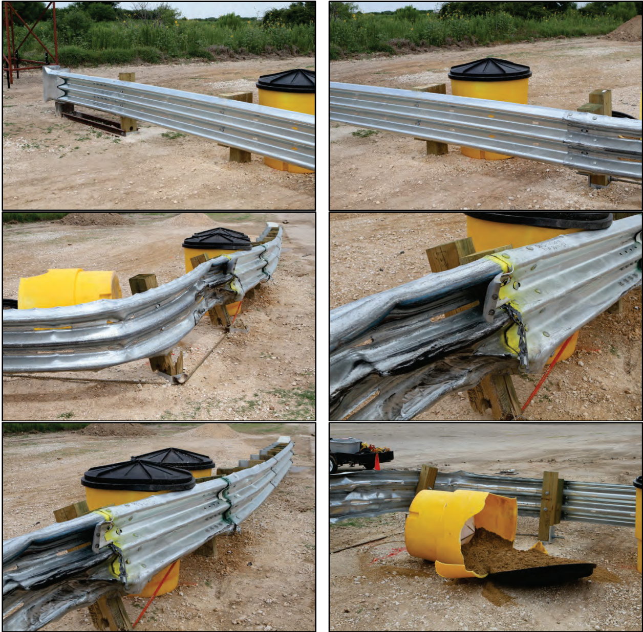
Figure 7.15. Installation after Test No. 467114-5.
