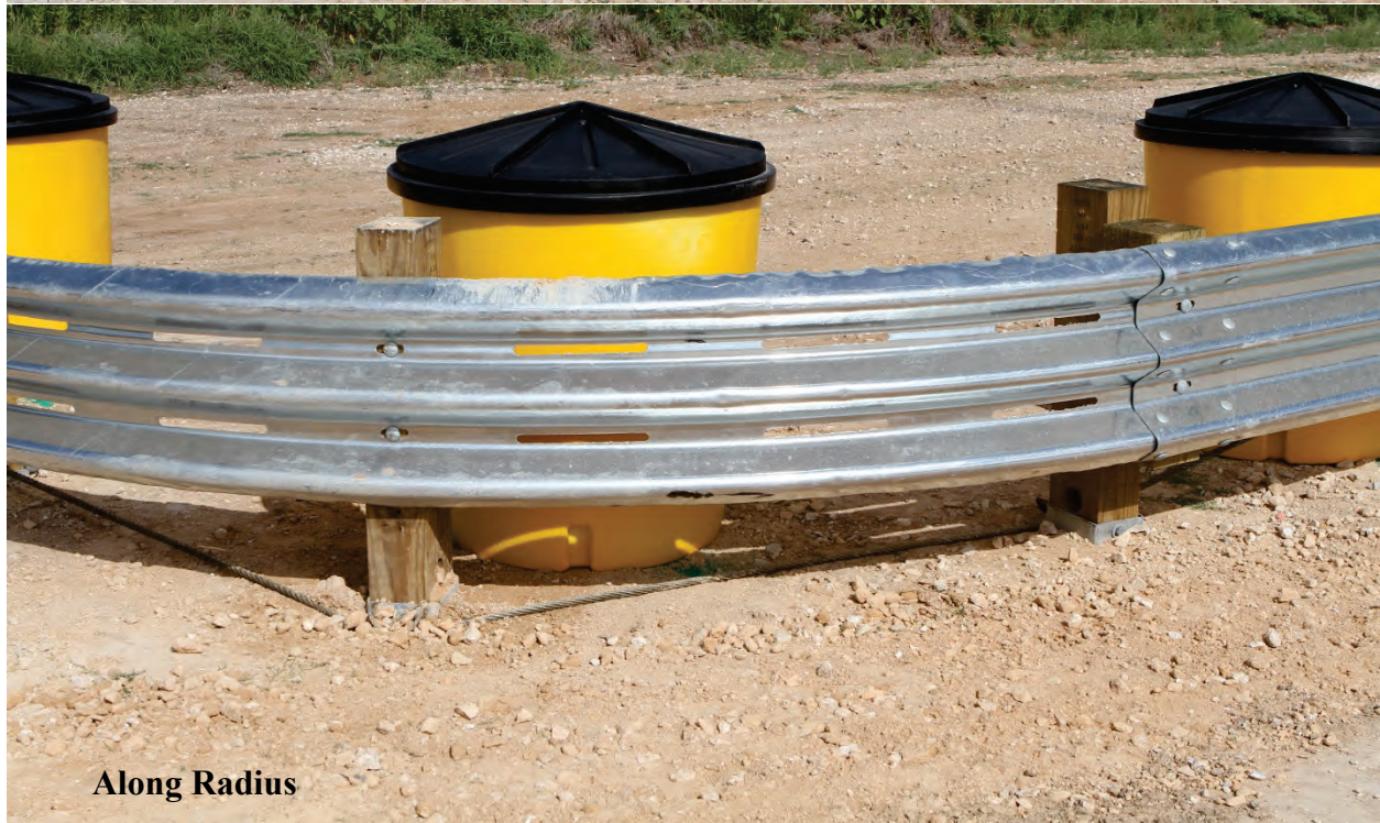
Figure 5.7. Short Radius Guardrail (Overall, Secondary Road, and Radius) prior to Test No. 467114-7.
