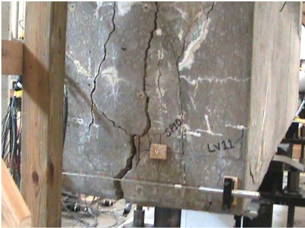
(c) At 498 kip (Just before Failure)
