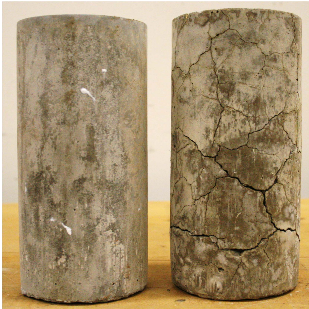
(a) Wet-Room Cured Cylinder
