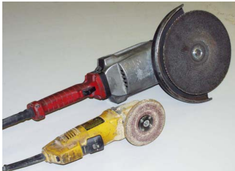
Figure 2-14. Typical disc grinders (Dexter and Ocel 2013)
