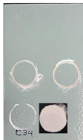
Figure: 4.36 Three-Coat Coating Pull-Off in As-Received Condition.
