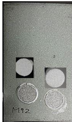
Figure: 4.33 Metallized Coating Pull-Off in As-Received Condition.
