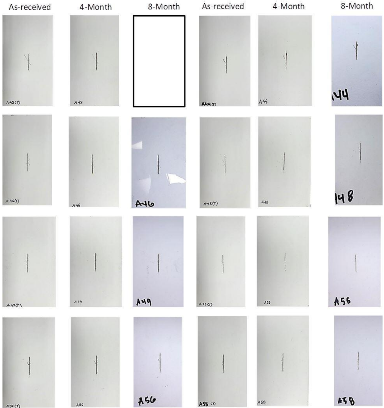
Figure: B.2 CPBC (Scribed) Samples Installed at Inland Test Site
