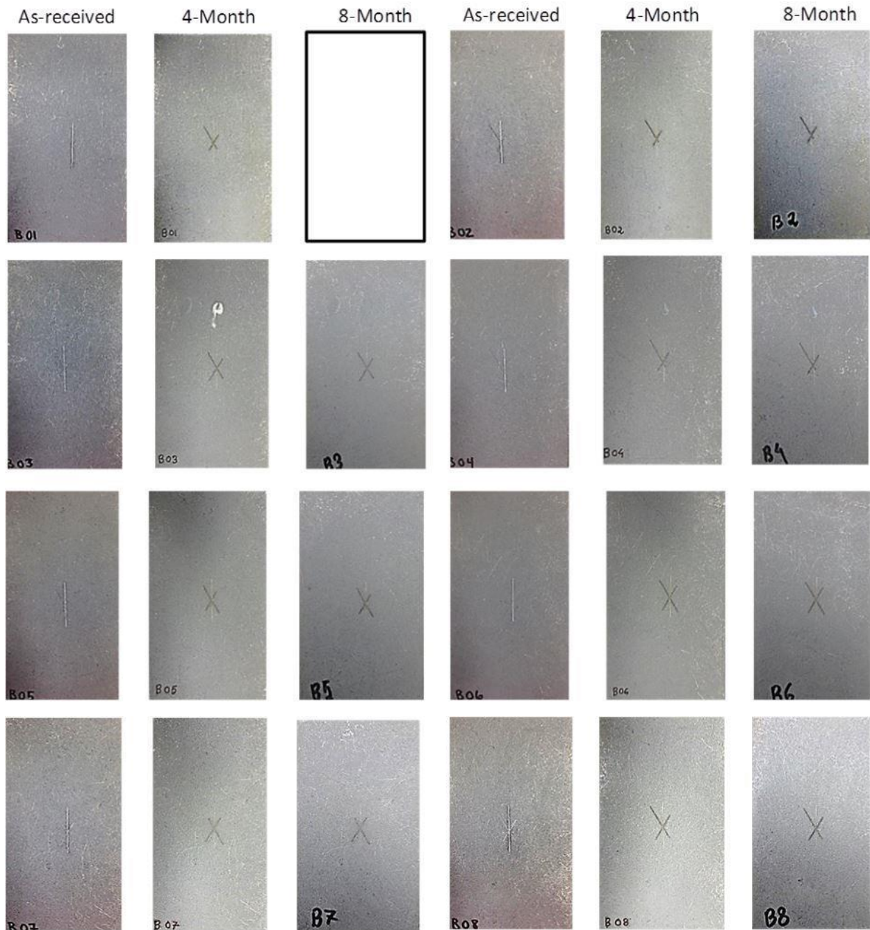
Figure: B.8 TDG (Topcoat A, Scribed) Samples Installed at Inland Test Site
