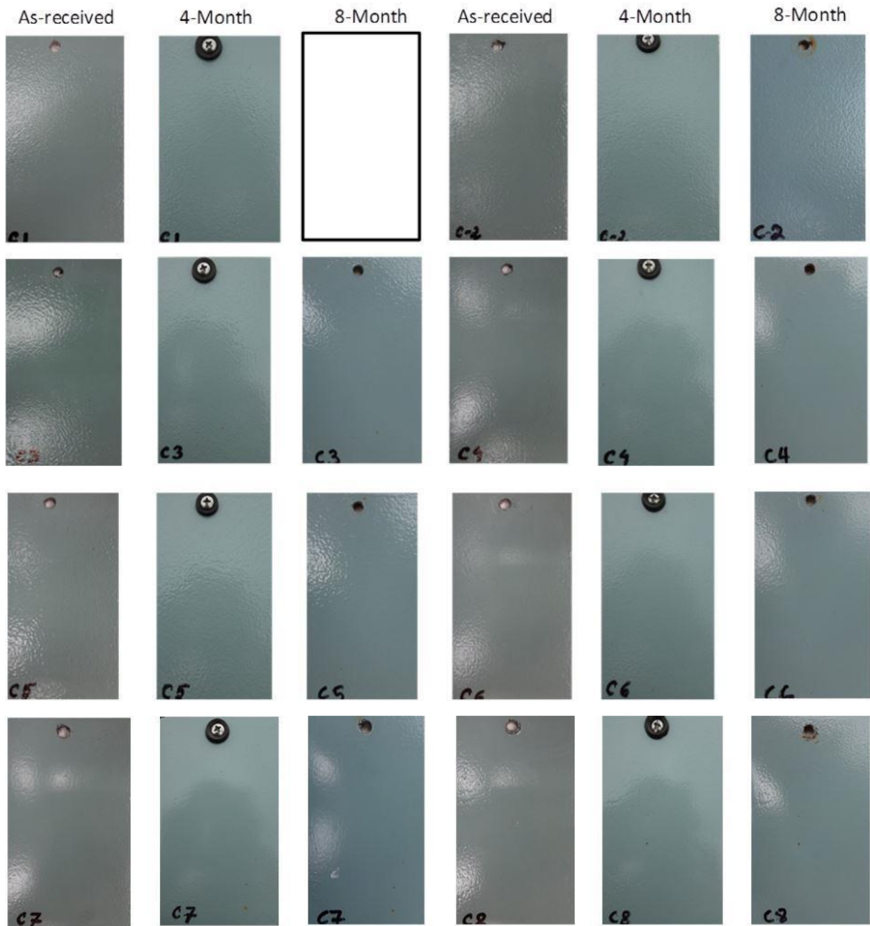
Figure: B.26 Three-Coat (Non-scribed) Samples Installed at Beach Test Site
