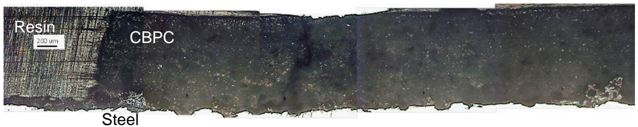
Figure: 4.40 CBPC Coating Micrograph after 4-Month Outdoor Beach Exposure.
