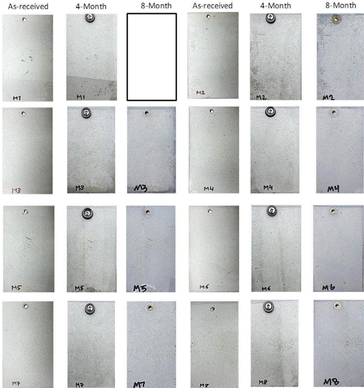
Figure: B.20 Metalizing (Non-scribed) Samples Installed at Beach Test Site
