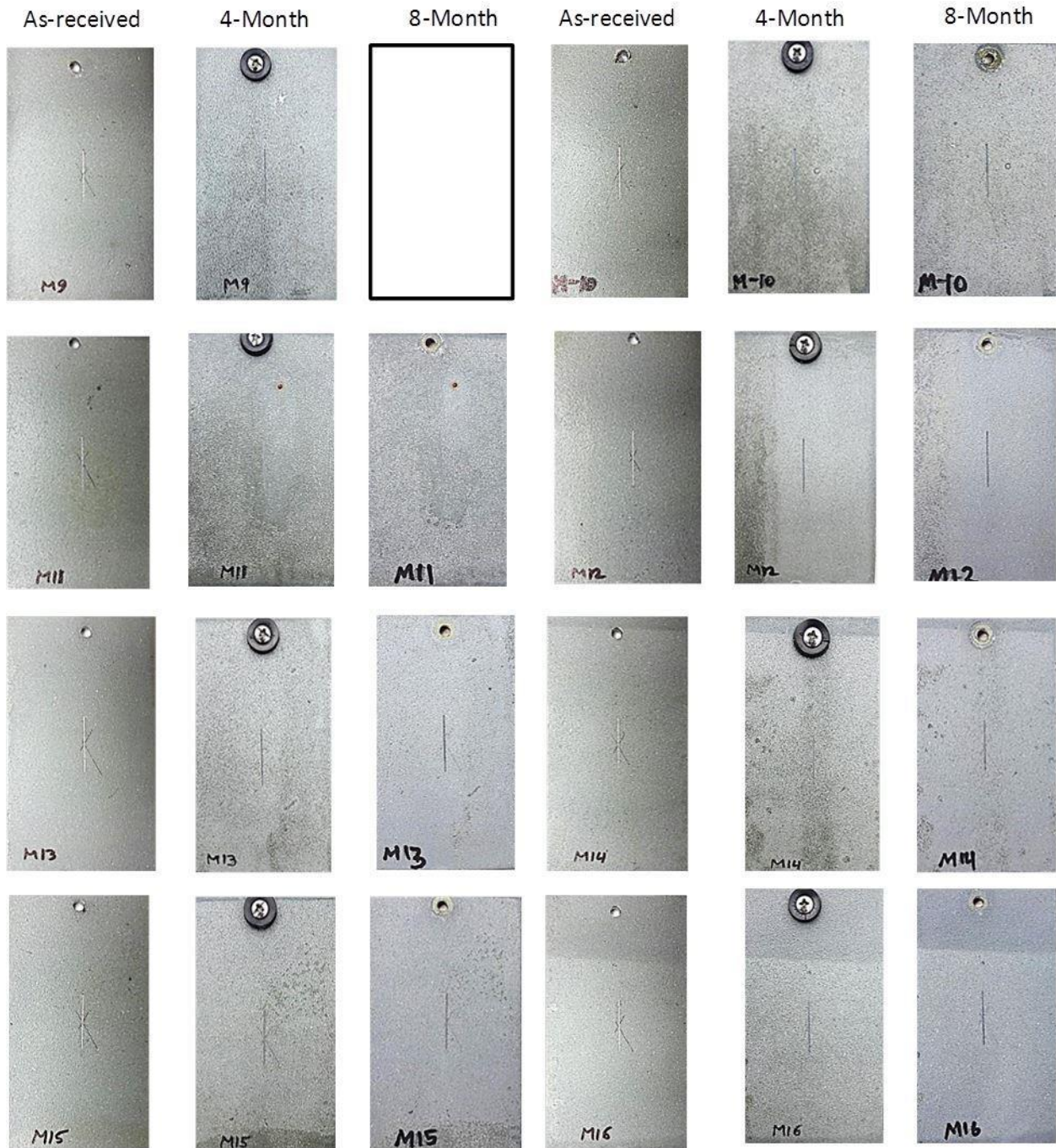
Figure: B.21 Metalizing (Scribed) Samples Installed at Beach Test Site
