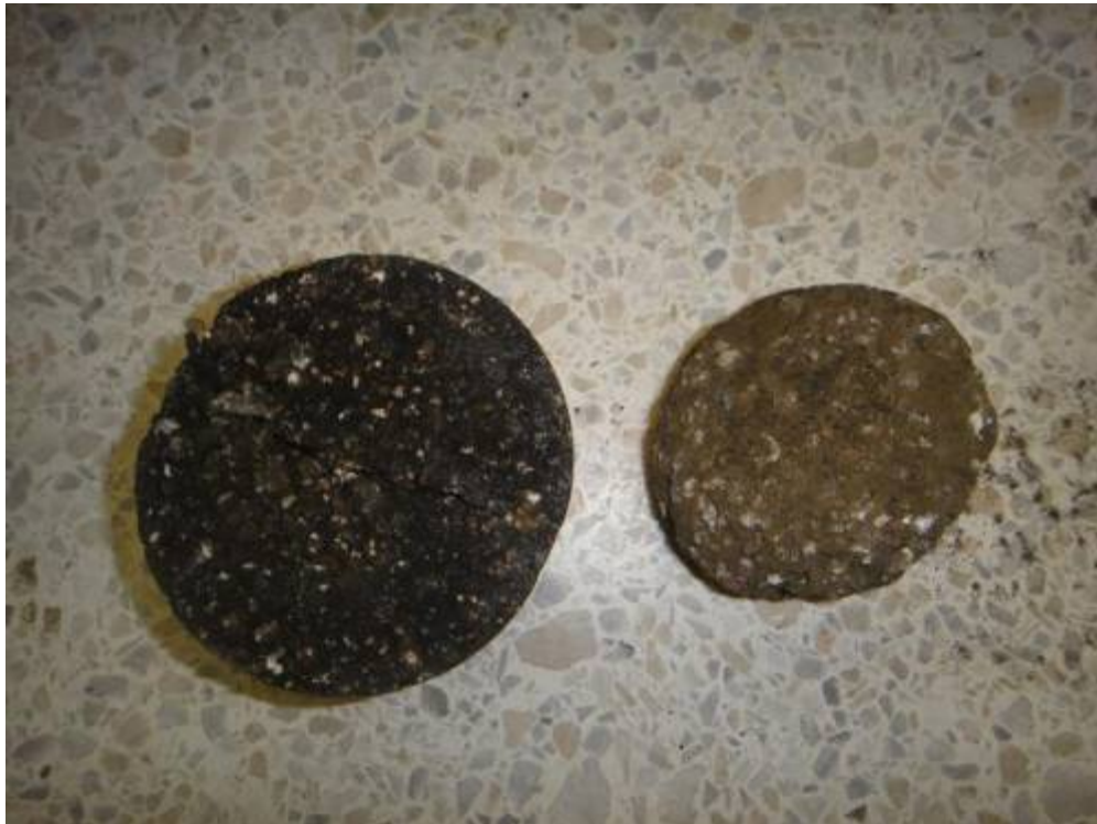
Figure 16. Texas Gyrotory LRA Specimen before and after Cantabro Test.
