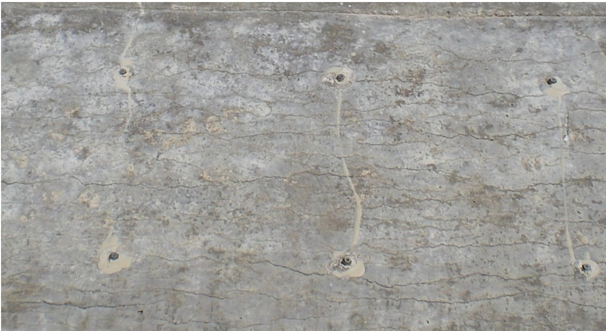
Figure 3-8. Typical Longitudinal Crack in Specimens.
