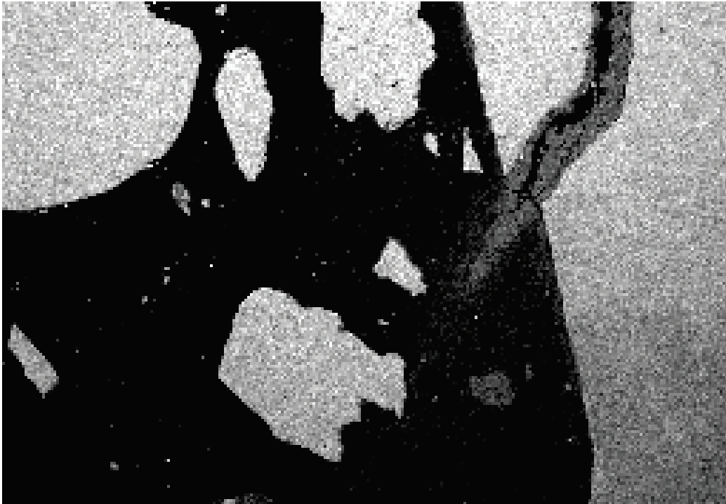
Sulfur dot map illustrating ettringite filled micro cracks associated with distress
