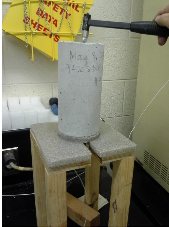
Figure 3-15 Free-free resonant testing.
