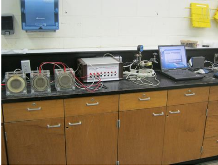
Figure 3-14 Rapid chloride permeability testing.
