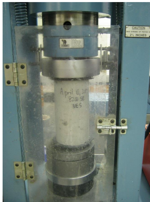
Figure 3-13 Compressive strength testing.
