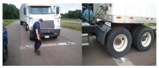
Figure 2.3 Weighing a CMV using pavement cut-outs
