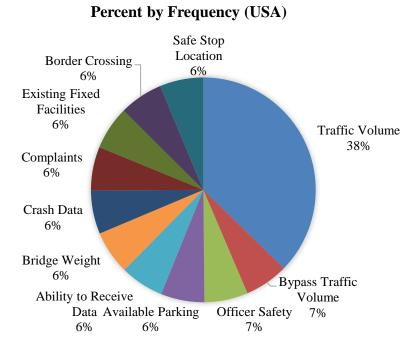
Figure 3.8 Criteria for selecting location of WIM sensor for mobile weight enforcement
