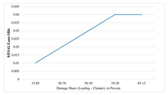
Figure 5.3 The impact of damage share proportions on unit pavement maintenance cost
