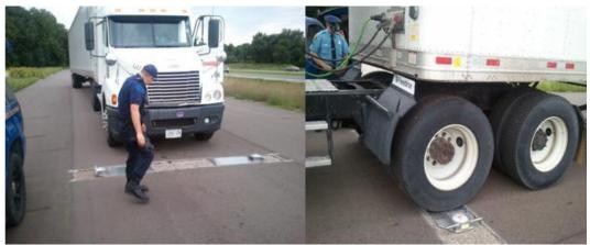
(b) Weighing and inspecting the truck
