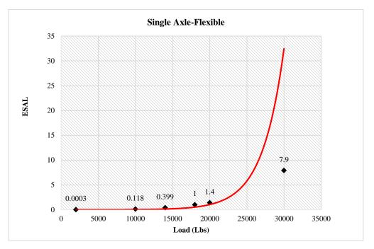
Figure 5.2 Single Axle Flexible Pavement ESAL
