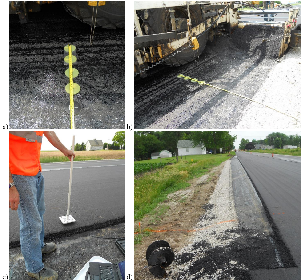
Figure 6.2. MEMS-based sensors embedded in IA 17 pavement: (a) 5 sensors laid on tack coat on intermediate course, (b) location of sensors in paving lane, (c) interrogation of sensors with RF antenna, (d) orange paint showing positions of first 3 embedded sensors
