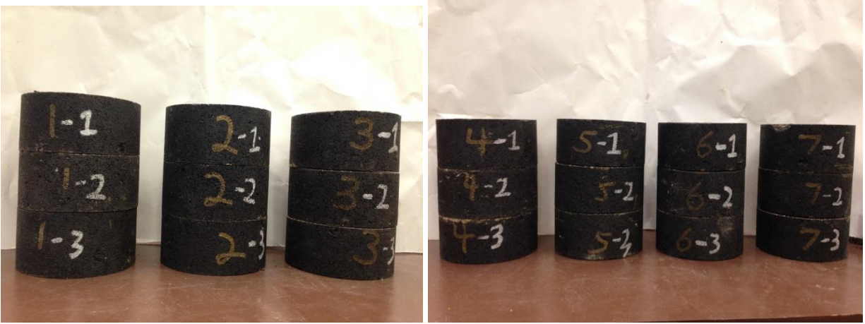
Figure 4.7. Photos of the seven calibration specimens for axial vs. IDT dynamic modulus tests
