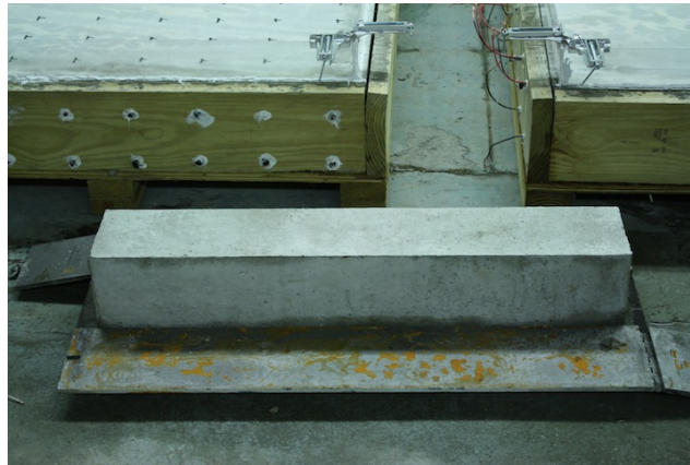
Fig. 11 Manufactured reinforced concrete beam specimen
