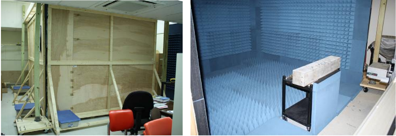
Fig. 15 An electromagnetic anechoic chamber at UML for testing the MRSS system
