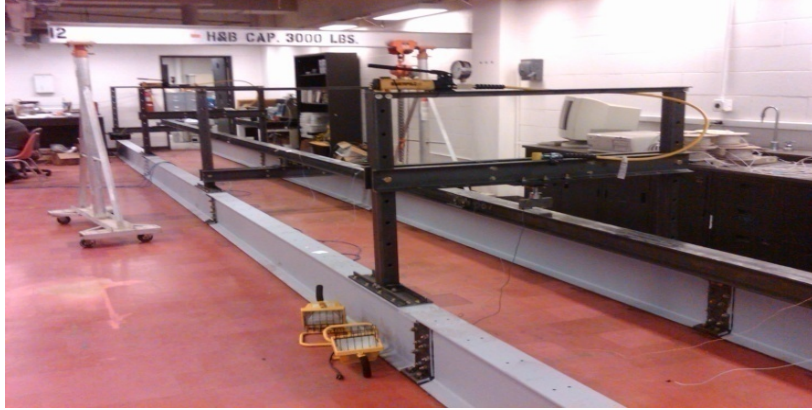
Fig. 9 Fabricated steel beam specimen
