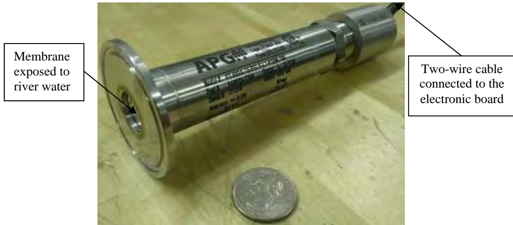
Figure 4.36 An APG PT-500 Pressure Sensor
