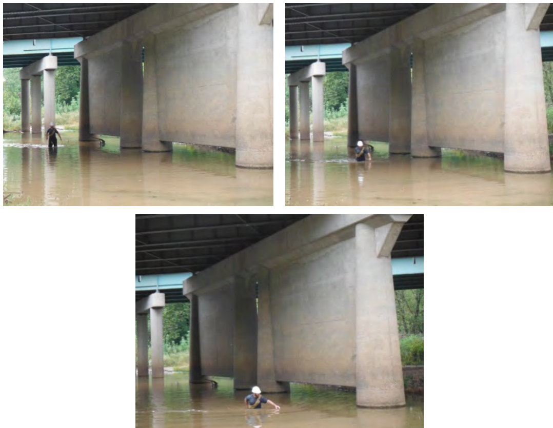
Figure 3.46 Manual Movement of a Prototype Smart Rock near a Bridge Pier
