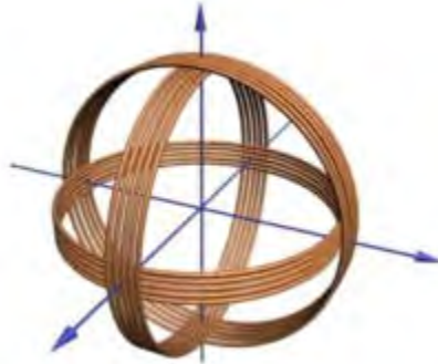
Figure 7.1 “Omnidirectional” Three-Channel Receiver Antenna for Each Smart Rock
