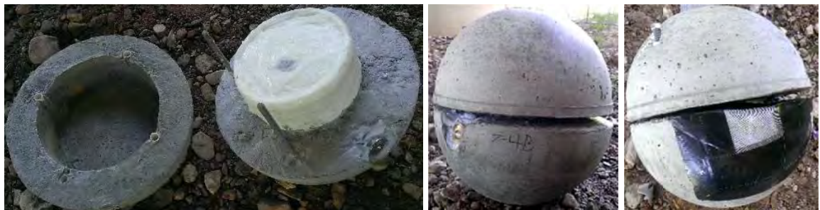
(a) Two Halves of Encasement (b) Complete Encasement (c) Sensor Protection Mesh
