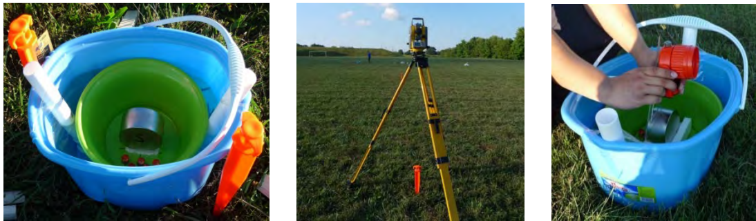
(c) Primitive APSS (d) Total Station for Positioning (e) Prism for Precision Positioning
