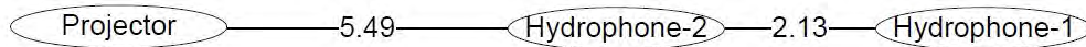
(b) Relative Locations of the Projector and Hydrophones with Distance in Meter
