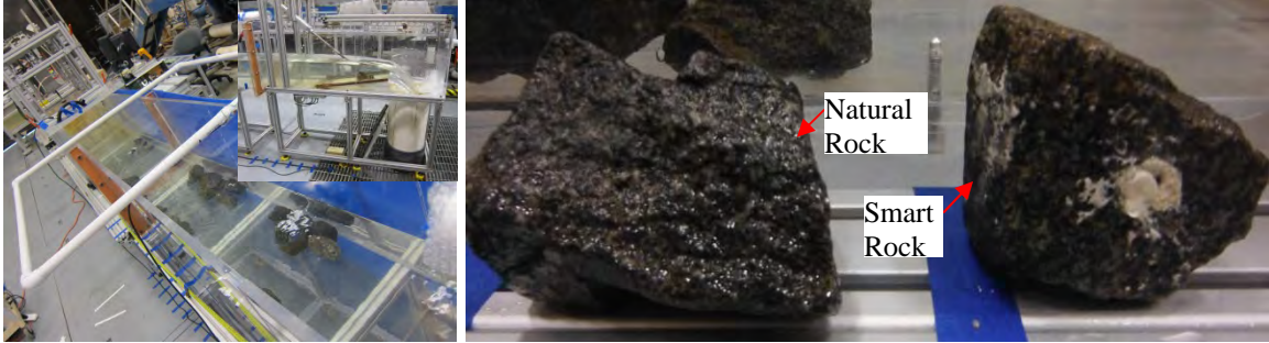
(a) Small Flume at TFHRC (b) Natural Rocks with and without an Embedded Magnet
