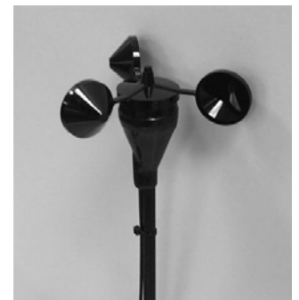
Figure 2: Attach Wind Speed Sensor to Mounting Pole
