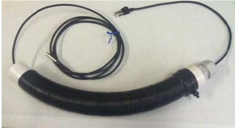
Figure 16. Onset temperature sensor with PVC jacket installed over smart sensor tube (Photograph provided by Mr. Tom Stalcup)
