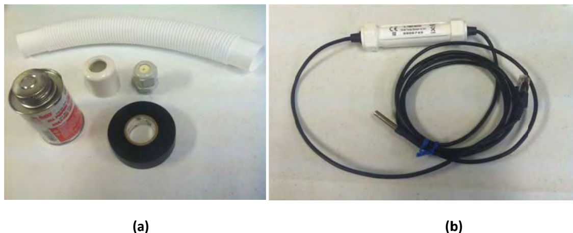
Figure 15. (a) PVC jacket materials (b) Onset temperature sensor without jacket
