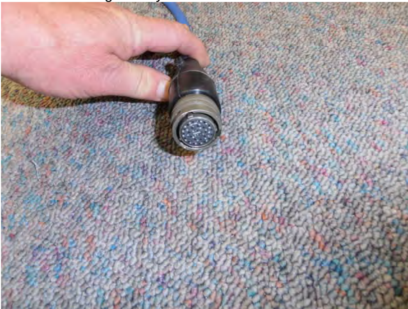
Thermistor String Military Connector with Overmould
