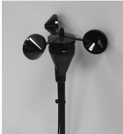
Figure 3: Attach Wind Speed Sensor to Mounting Pole
