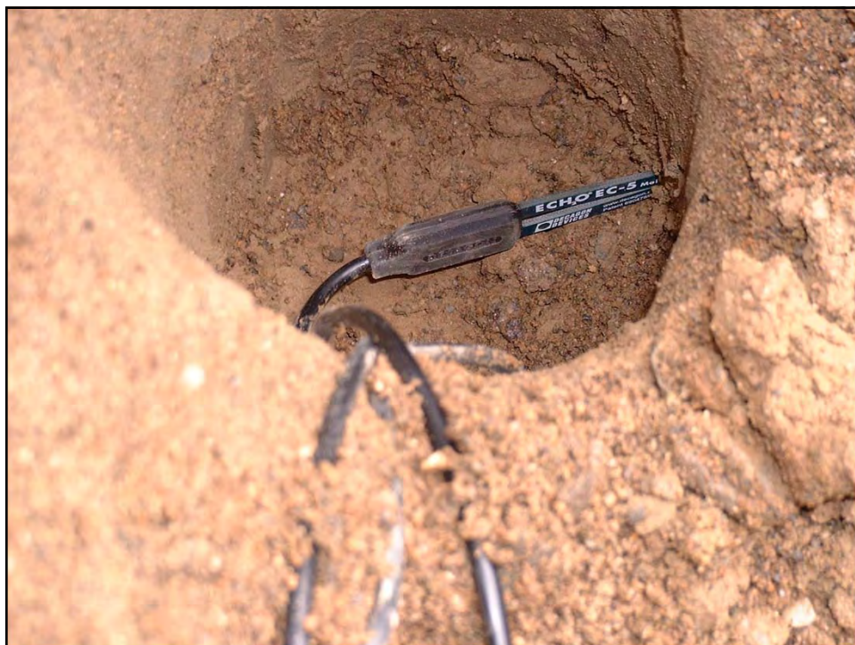
Fig E-24. Third Soil Moisture Sensor from Bottom of Borehole
