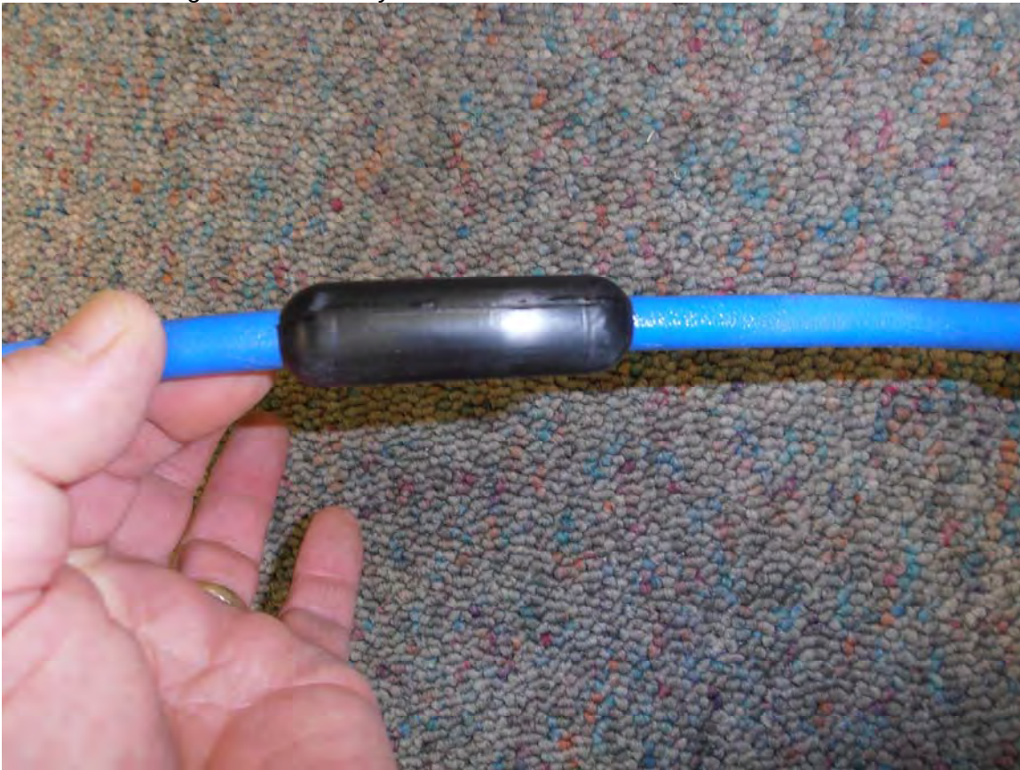
Thermistor String Thermistor Polyurethane Shot
