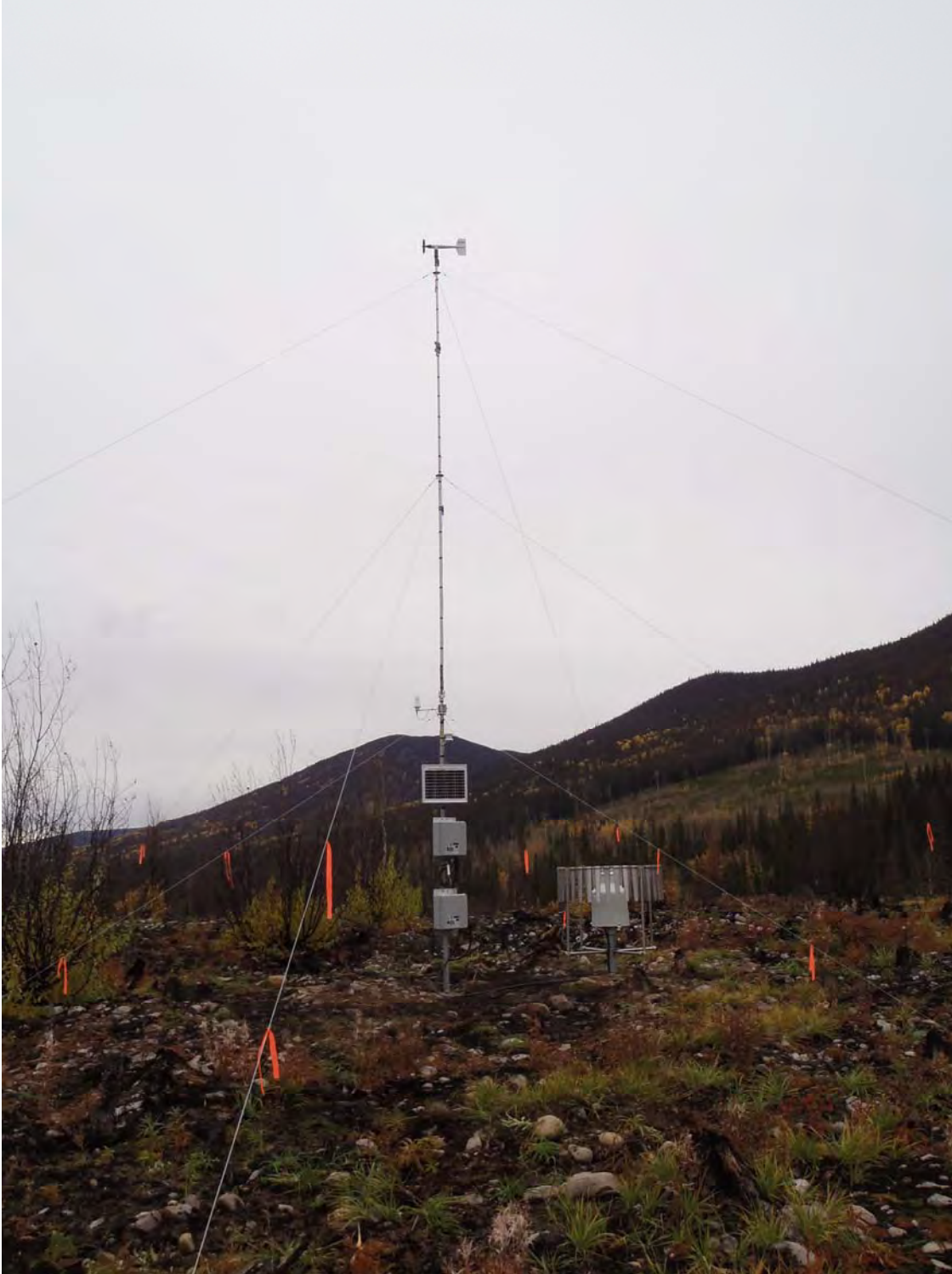
Example Iridium Climate Station with 30 Foot Pop-Up Mast
