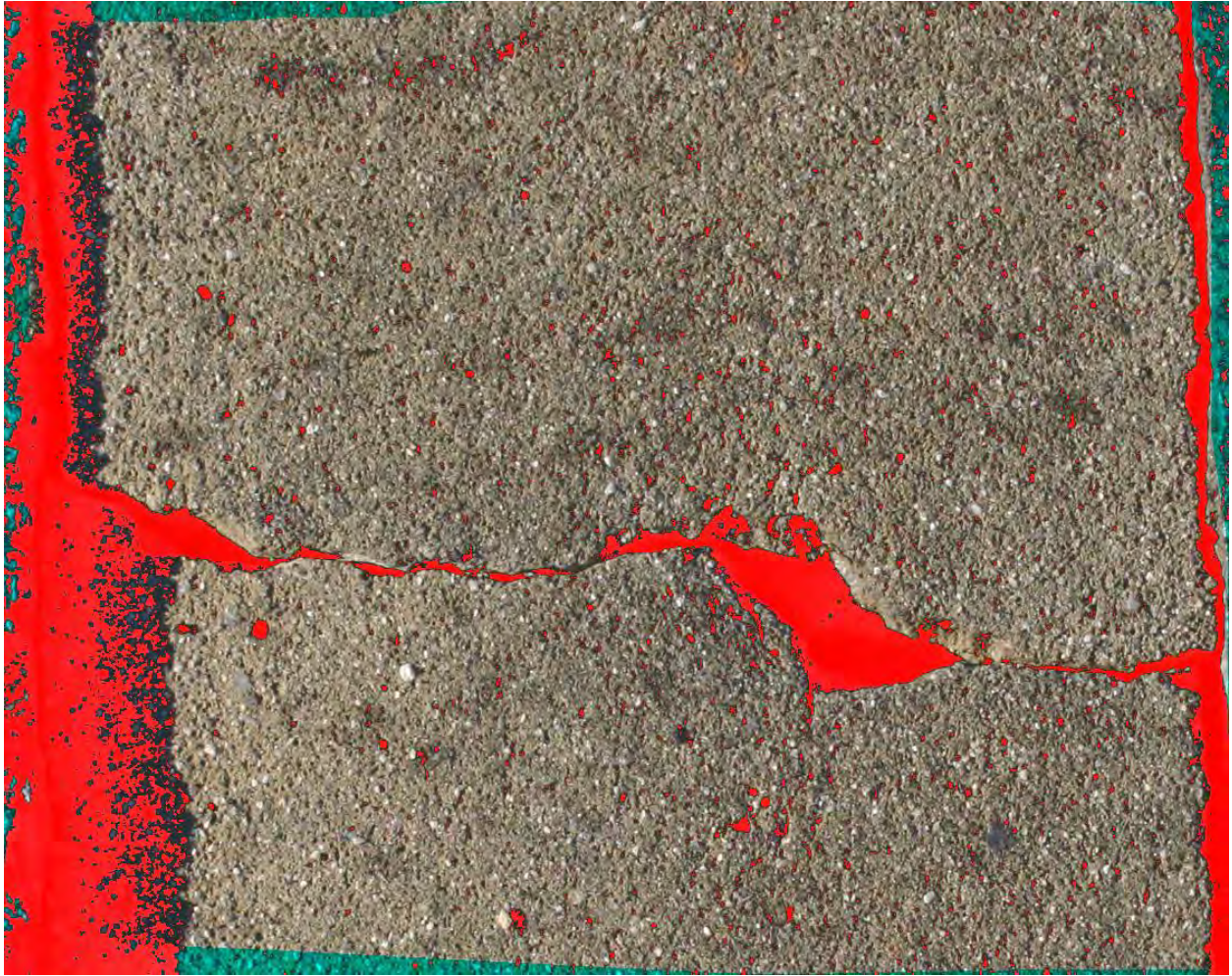
B.1.5: Original image of the area of study being marked with major cracks in red pixels
