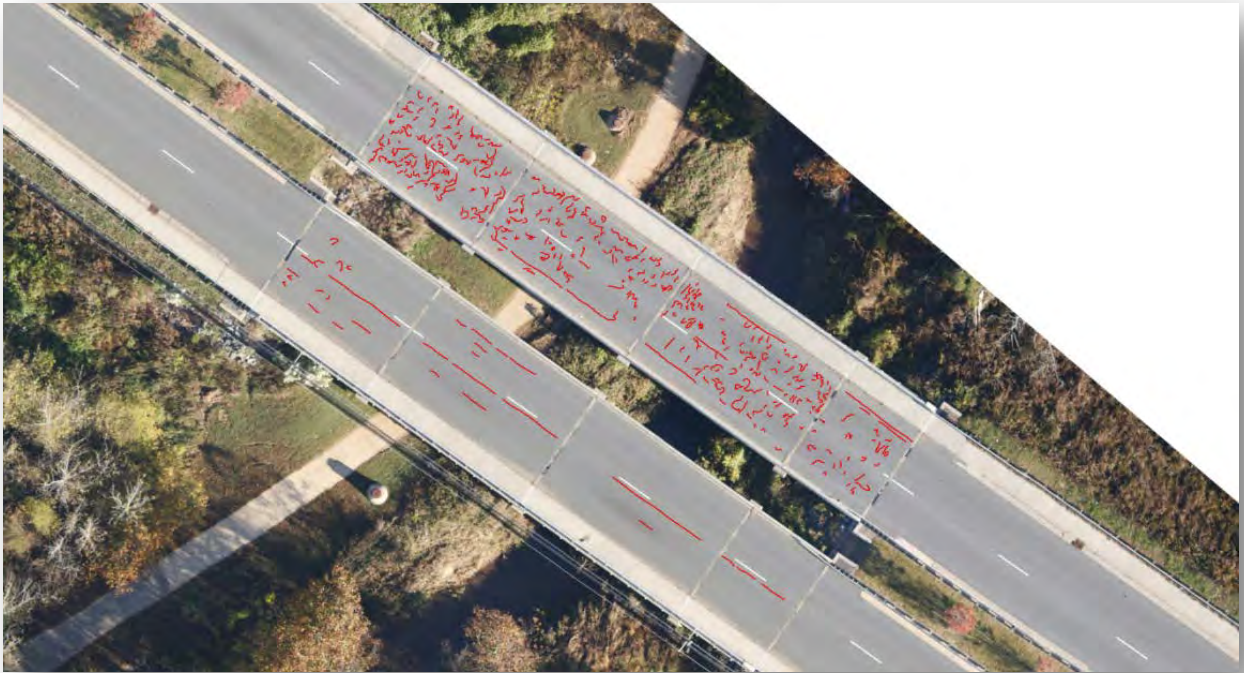
Figure C.7.2: Bridge NO. 590084 Crack Image
