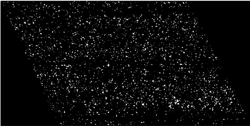
Filtered Image of Minor Cracks
