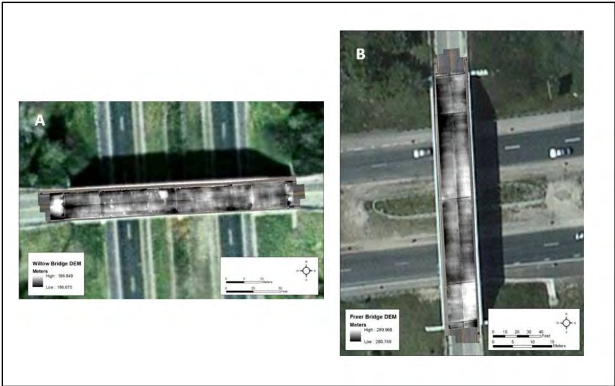
Figure 4-17: DEMs generated by 3DOBS of Willow Road (A) and Freer Road (B) bridges.
