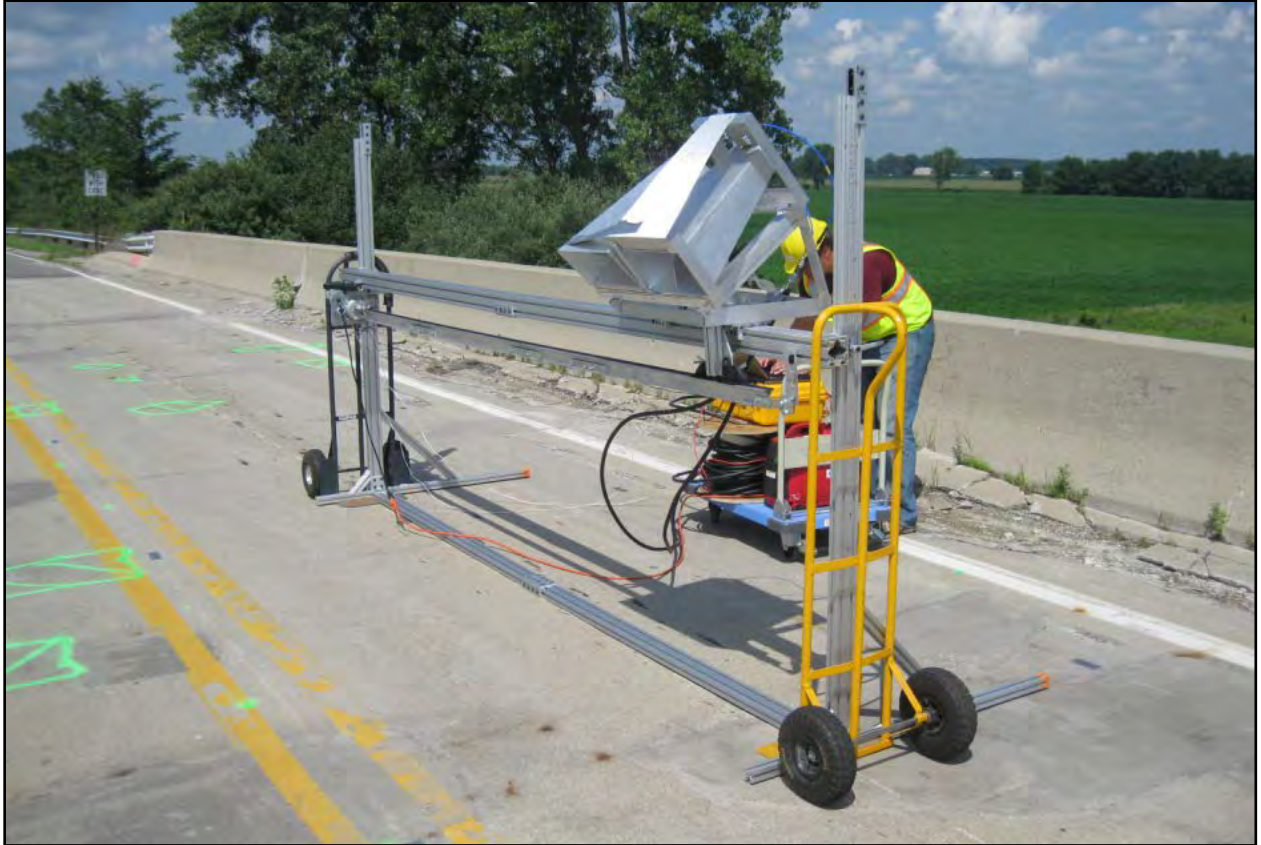
Figure 10-4: More "mobile" translator apparatus and RaDAR equipment, which could be adapted for moving vehicle-based deployment.
