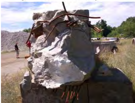
Figure 10-12: Photographs of the salvaged box beam used in the 3D GPR imaging experiments.
