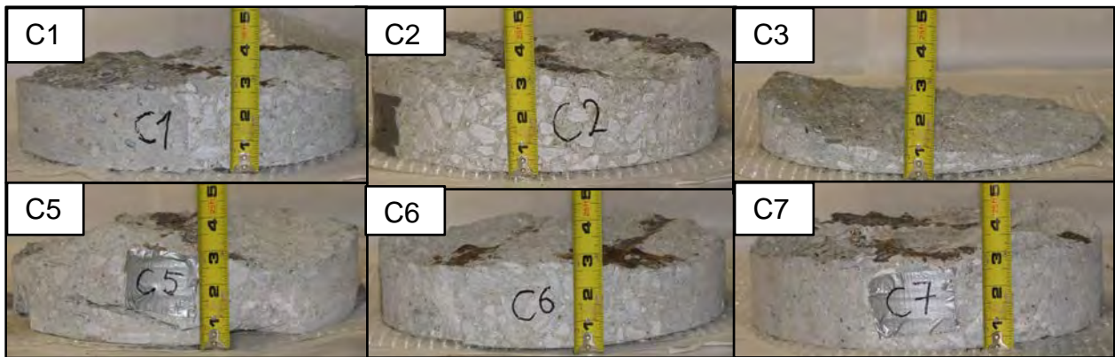
Figure 8-22: Six of the 10 cores extracted from the Mannsiding Road bridge deck.
