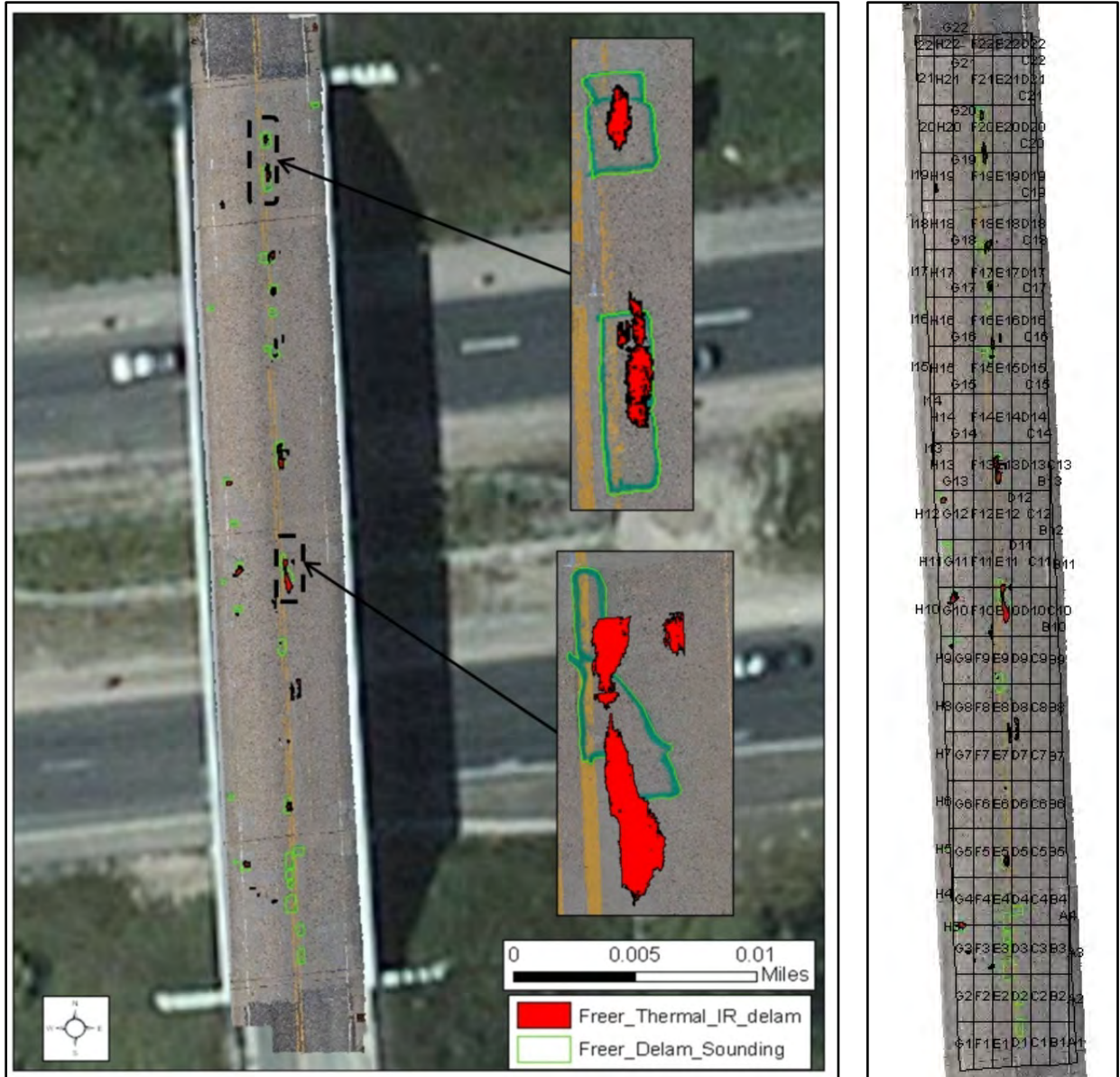
Figure 8-14: Thermal IR and sounding delamination map and the virtual grid pattern over the Freer Road bridge displayed on ArcGIS.
