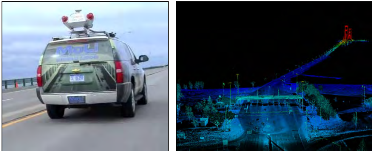
Figure 7-3: SSI Surveying Solutions Mobile LiDAR (MoLi) truck and LiDAR scan of the Mackinac Bridge and toll plaza.
