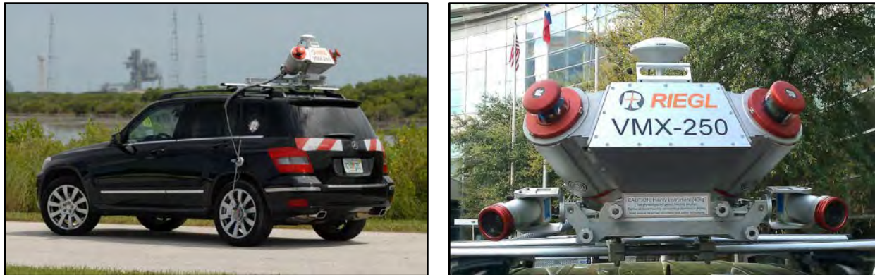
Figure 7-23: The VMX-250 scanner mounted on an SUV. Image on the right shows a close-up of the scanner heads, GNSS receiver, and Processing/Inertial Navigation Unit.
