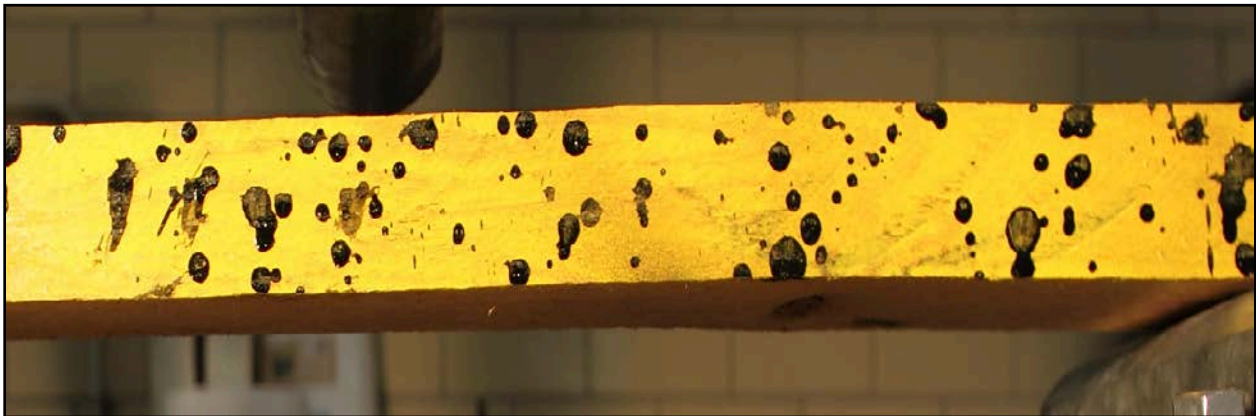
Figure 9-8: Wood Beam with speckle pattern.
