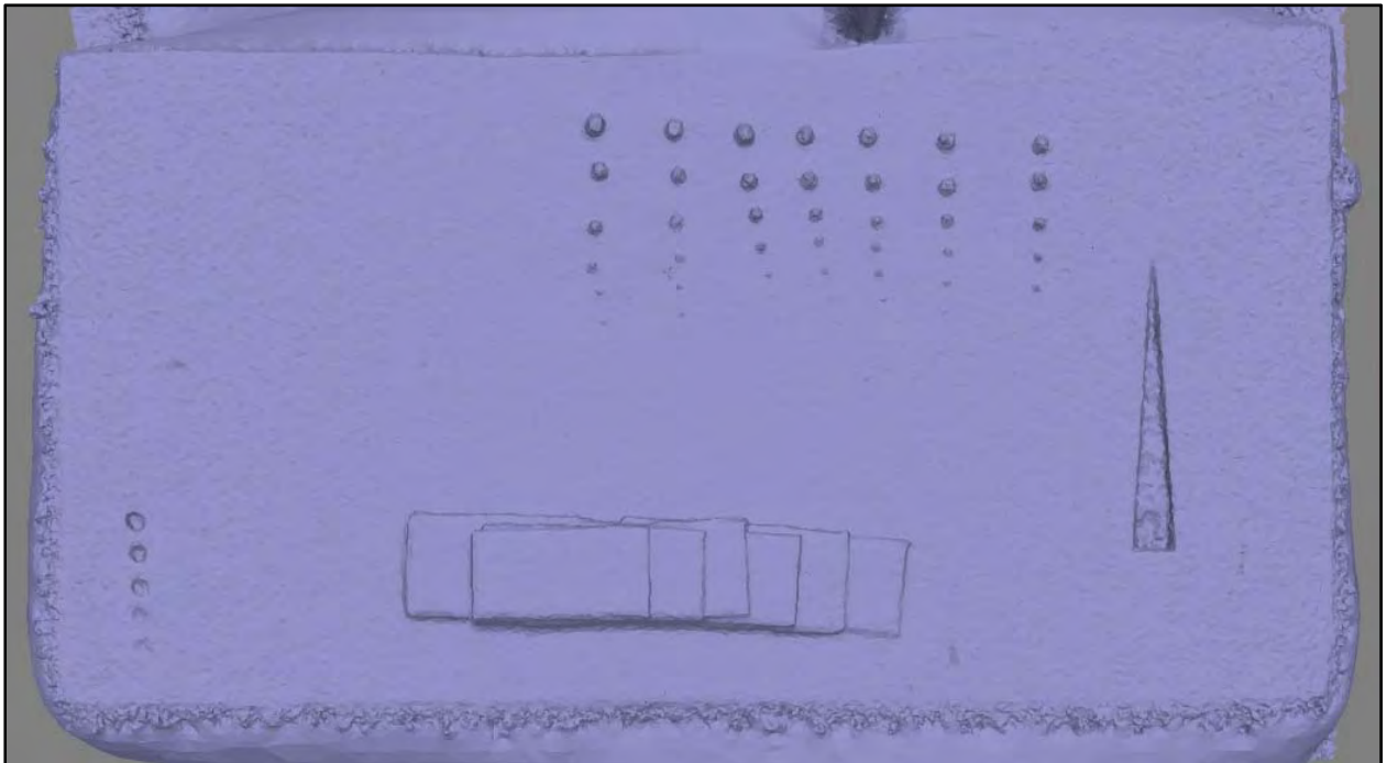
Figure 4-2: The resulting PhotoScan model. A total of five photos were used to generate this model.
