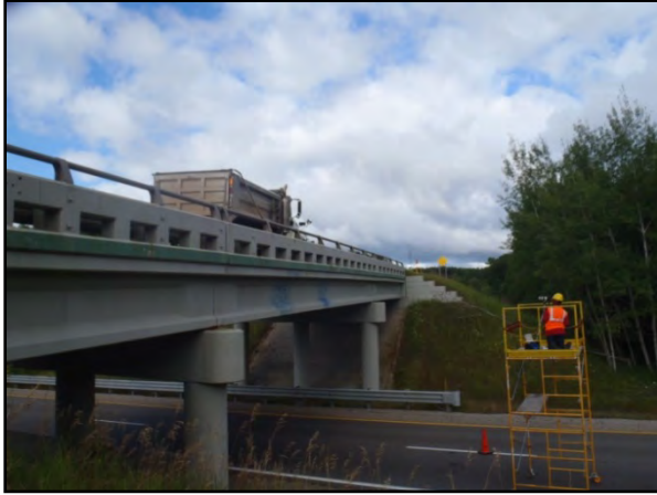
Figure 9-13: Load truck going over bridge (left) and close-up of camera and tripod setup on scaffolding (right).
