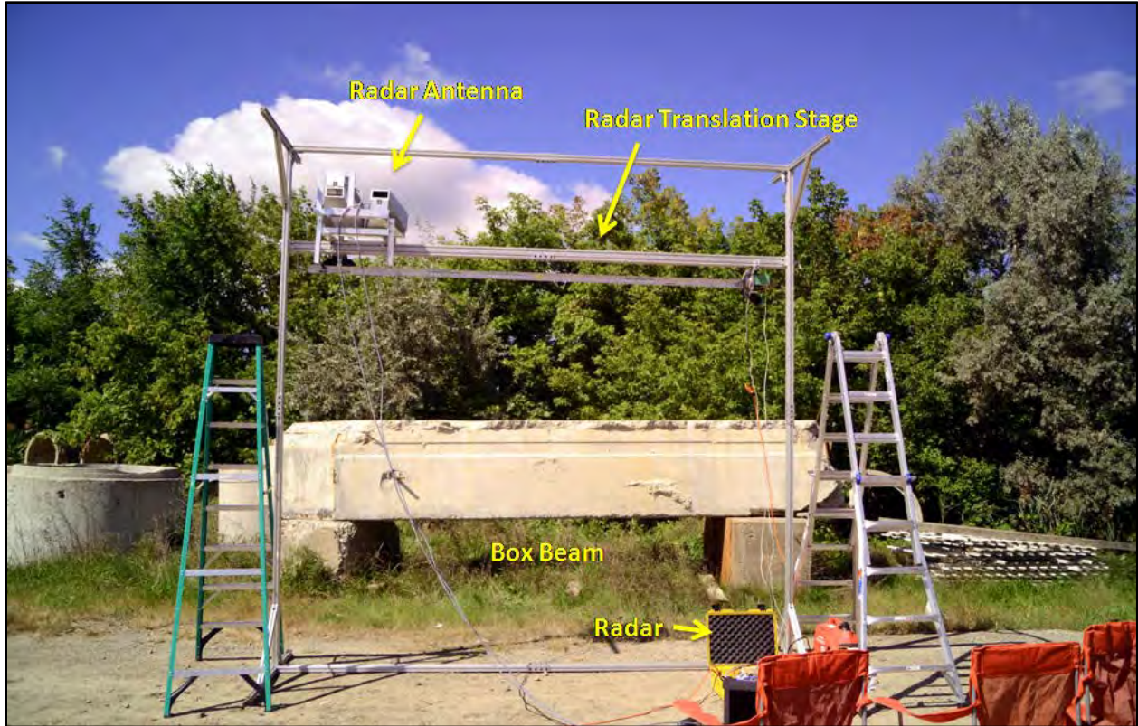
Figure 10-13: Portable imaging RaDAR mounted on a 2D Translation stage parallel to side of Salvaged concrete box beam at measurement site at Oakland County Road Commission site in Waterford, MI.
