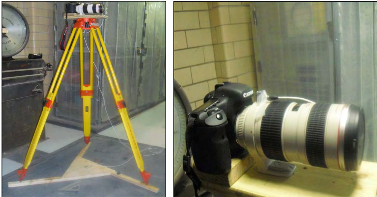
Figure 9-23: Camera on stable tripod (left) and detailed of mounted accelerometer (right).
