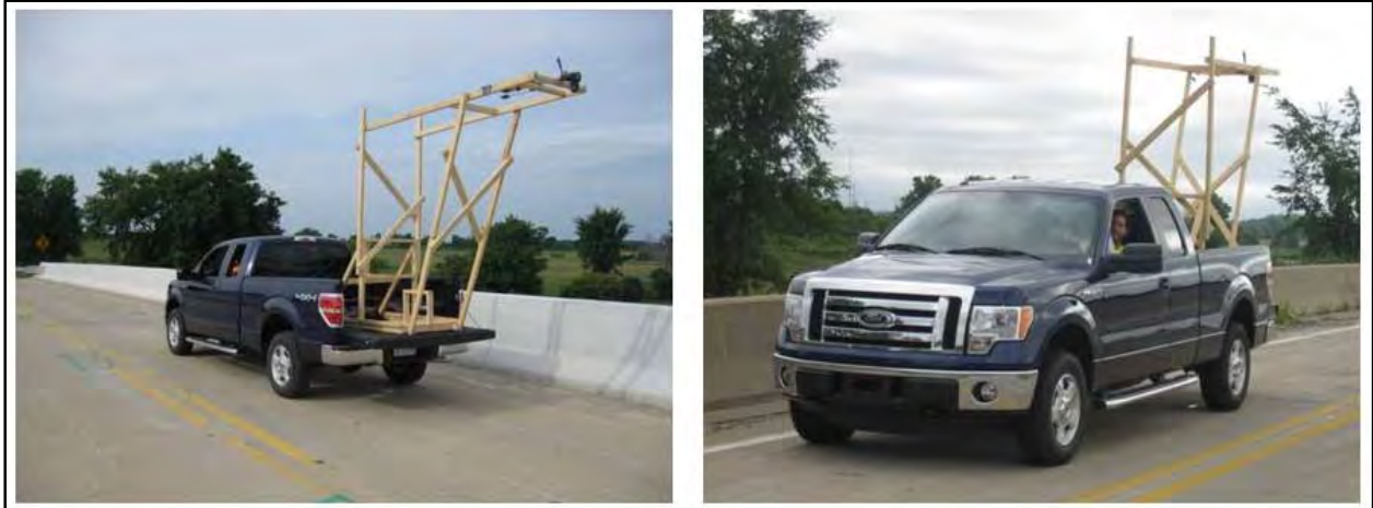
Figure 4-5: 3DOBS vehicle mount in the bed of a pickup truck. The image on the left was taken on Willow Road bridge and the one on the right on Freer Road bridge.
