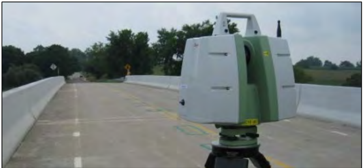
Figure 7-2: An example terrestrial LiDAR scanner used to collect 3D data of the project’s demonstration bridges. The unit was deployed by the project’s Michigan DOT partners.
