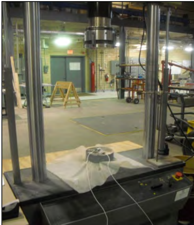
Figure 9-20: Accelerometers on the 810 Material Test System.
