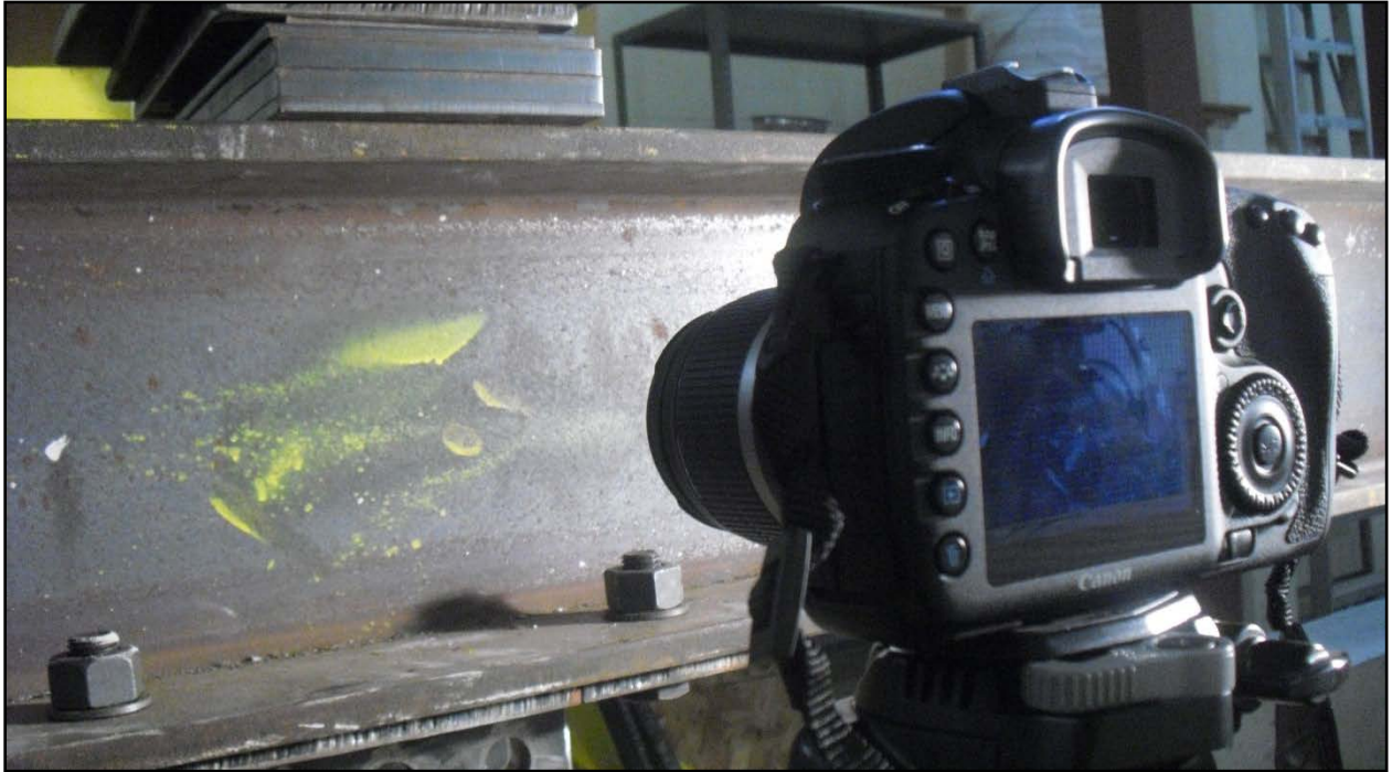
Figure 9-9: DIC Setup for steel W shape (I beam).
