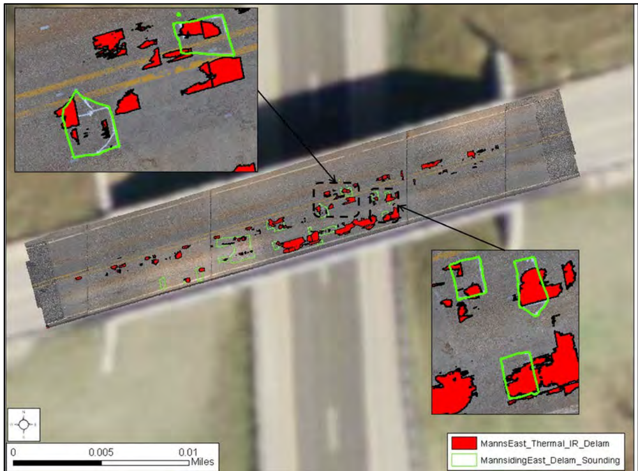
Figure 8-17: Thermal IR delamination map and sounding delamination map of Mannsiding Road bridge displayed in ArcGIS.
