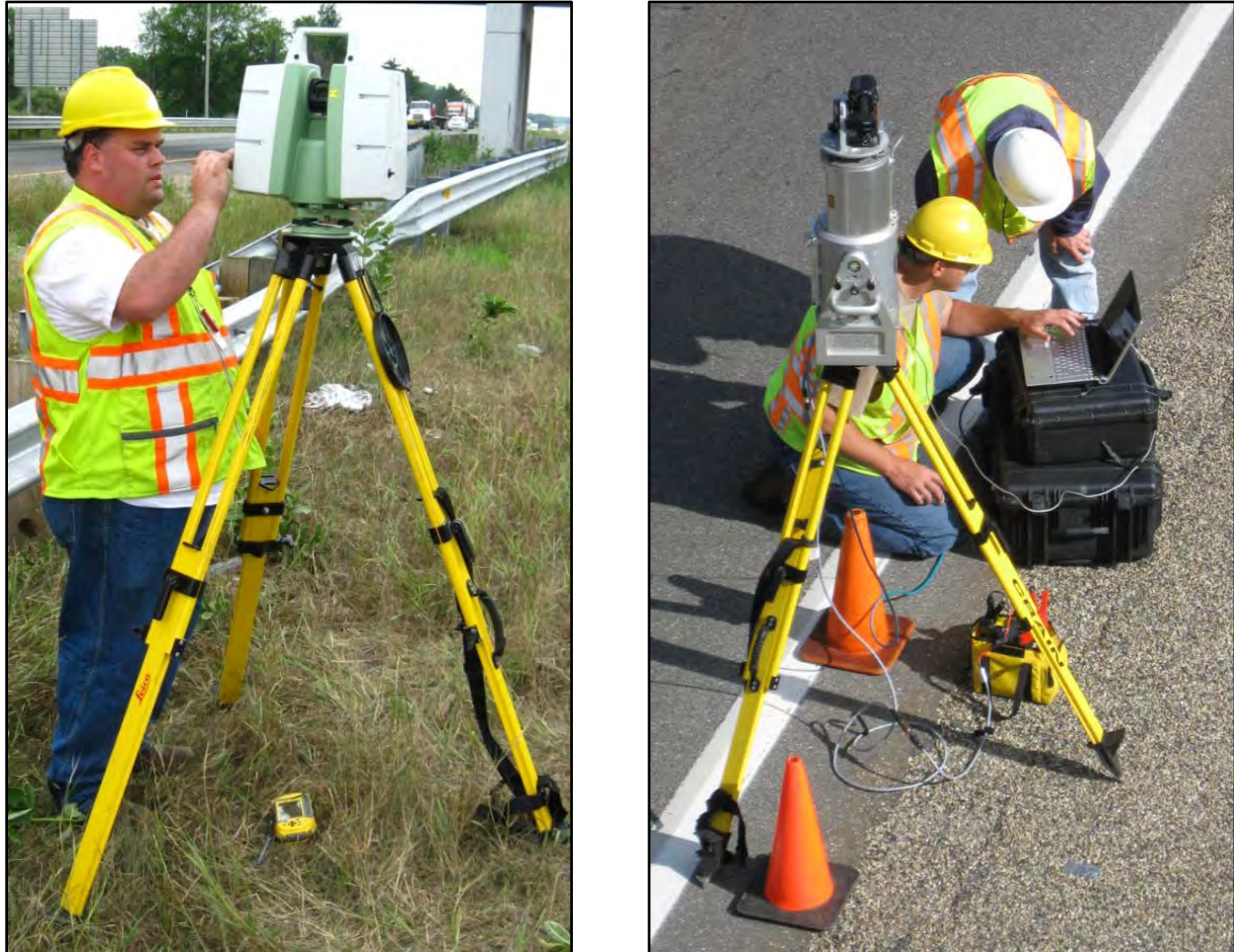
Figure 7-4: Typical terrestrial LiDAR units; MDOT’s ScanStation C10 and MTU’s Riegl LMS-Z210ii.
