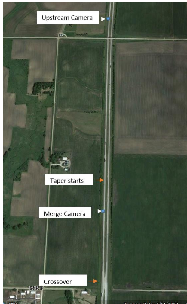
Figure 9. Camera placement for I-35 work zone
